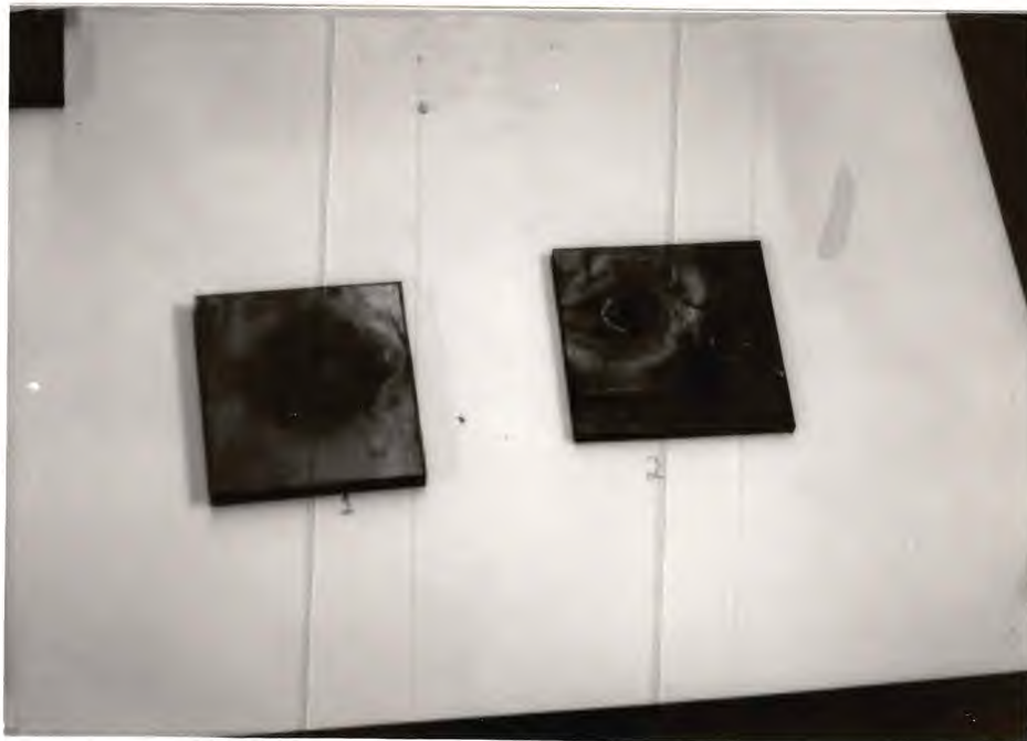
Fig 20 Effect of heating time on Waterjet piercing.
