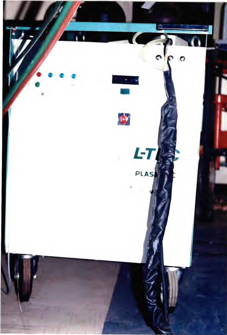
Fig 9. The Plasma Arc Cutting system
