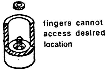
(a) Ensure Adequate Access for Part Insertion
