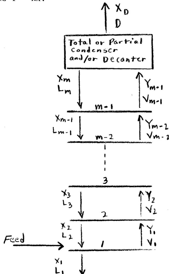
The Stage 2 component balance (feed is on Stage 1) is
