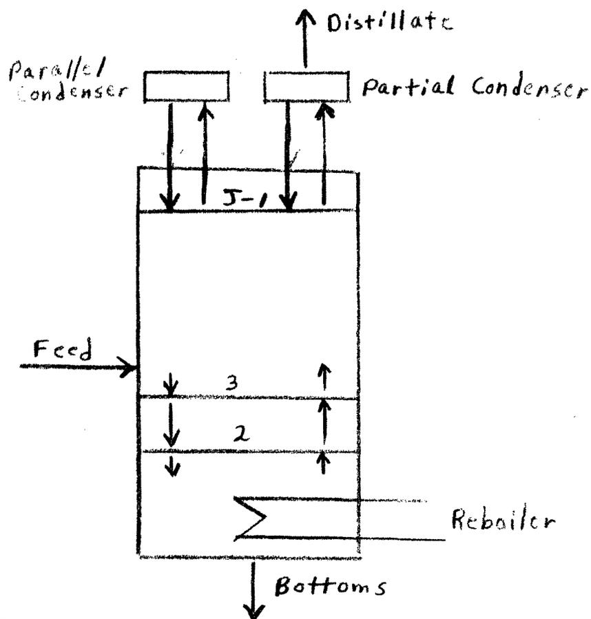
To further illustrate the need for a parallel condenser, consider the following development which solves for  $L(J)$ , the liquid from the partial condenser, from an enthalpy balance on the last stage, whereas equation (12) solves for  $L(J)$  from a material balance.
