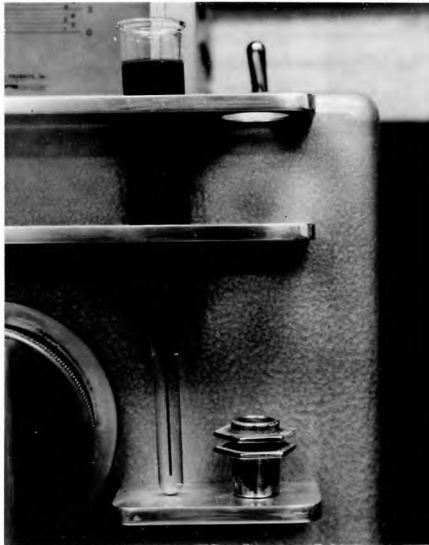
FIGURE 4. FEEDING CHAMBER AND CENTRIFUGE TUBE
