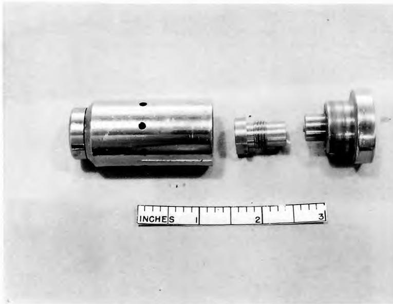
FIGURE 8. FUZE HOUSING AND LOADING FIXTURE ASSEMBLY
