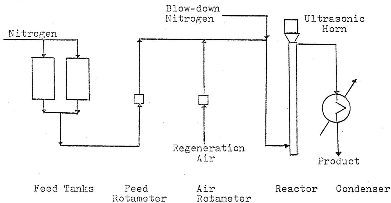
an ultrasonic horn. A heat exchanger is included to condense the product. Detailed specifications of all equipment have been described by Lintner and are contained in his Doctoral dissertation (1973). Lintner's work showed that:
