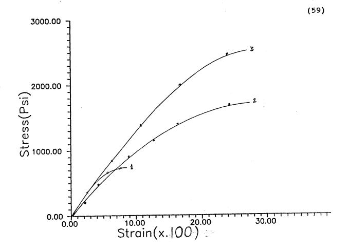
Fig.3.1 Stress(Psi) vs Strain (in/in) for Franklin fiber (Whisker fiber) (1) 43%, (2) 20% and (3) 15%.
