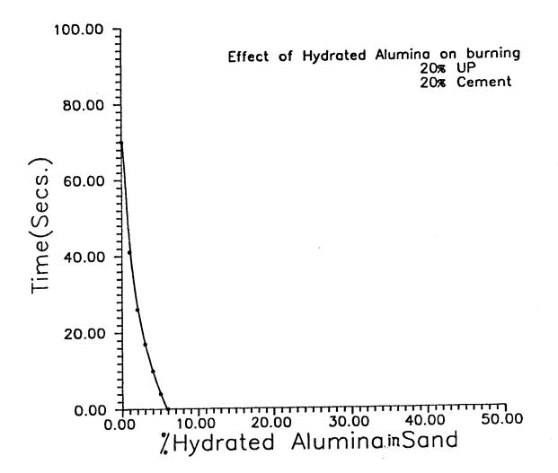
Fig.3.18 Effect on time of burning of PPCC, replacing sand by Trihydrated Alumina.
