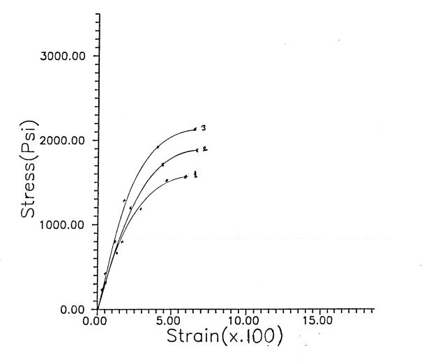
Fig.3.3 Stress(Psi) vs Strain (in/in) for Terra alba (1) 15%, (2) 20% and (3) 25%
