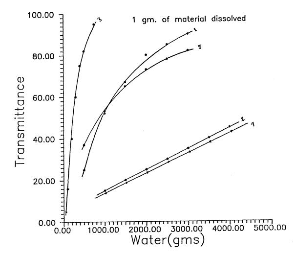
Fig.3.8 Transmittance for (1) Franklinfiber (2) Trihydrated Alumina (3) Terra Alba (4) Calcium Carbonate (5) Portland cement, when added (1 gram) in various amounts of water.
