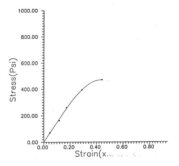
Fig.3.7 Stress(Psi) vs Strain (in/in) for Control sample 3.
