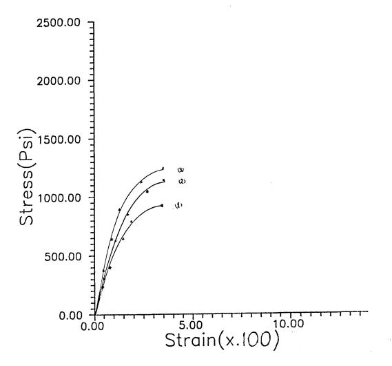
Fig.3.4 Strss(Psi) vs Strain (in/in) for Calcium carbonate (1) 15%, (2) 20% and (3) 25%.
