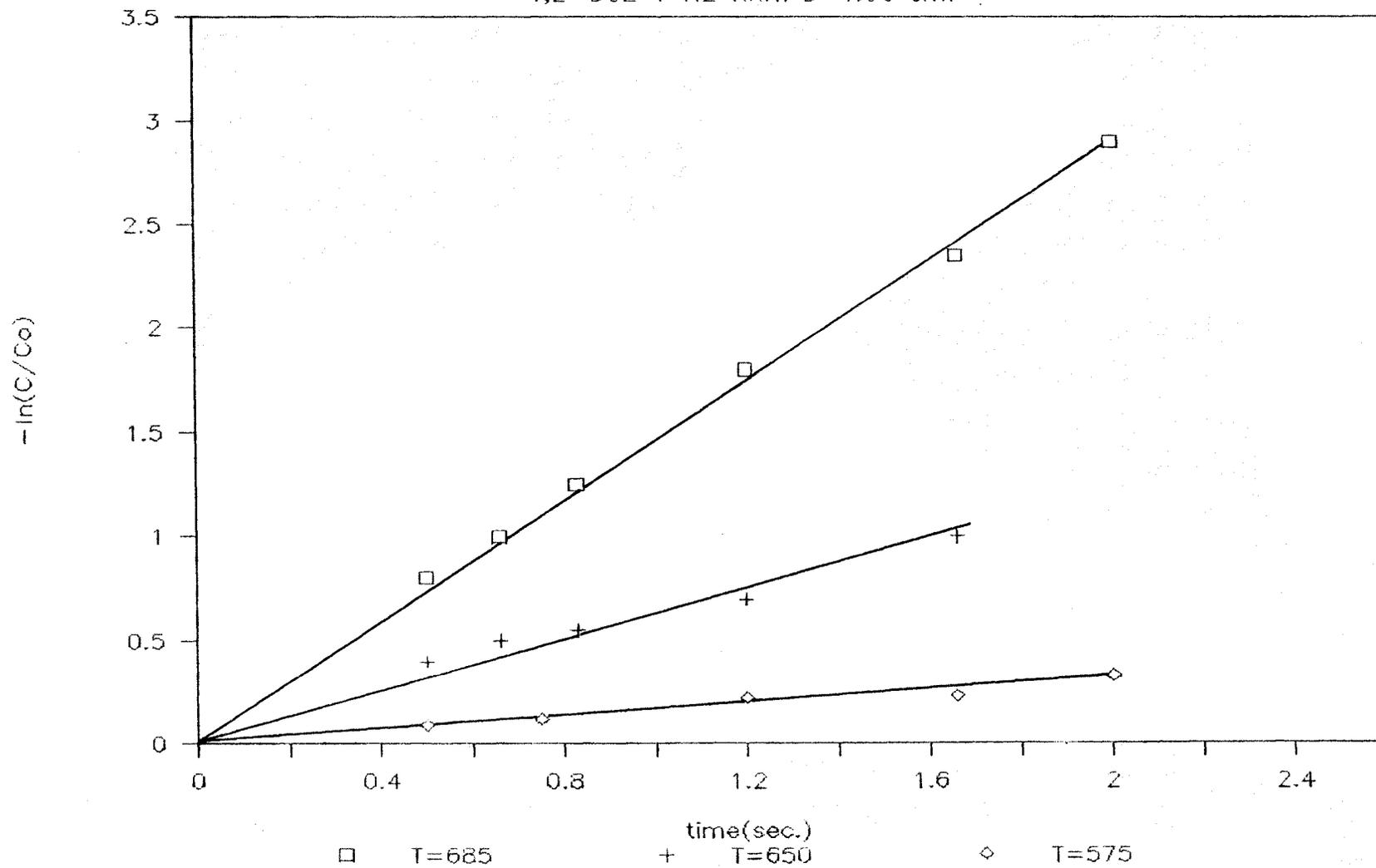
high conversion initiation achieved by this reaction. The conversion of 1,2-dichloroethane at these temperature range and residence time of 2.0 sec. are 30%, 55% and 85% respectively. At higher temperatures, the conversion becomes too high for meaningful kinetic study.
