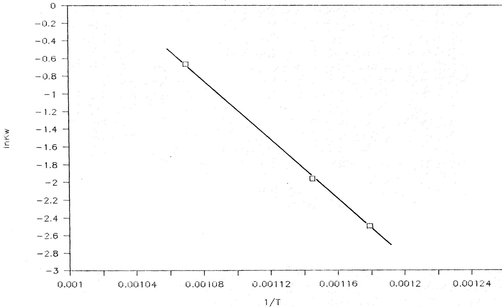
Figure 7: Arrhenius Plot for Kw
