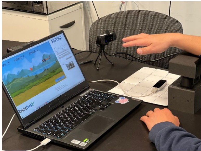
Figure 6.3 HoVRS system set up includes laptop, infrared motion capture camera, arm support, and video conferencing camera.
