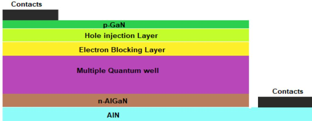
**Figure 2.3** Schematic Diagram of the Simulated AlGaN UV LED at 255nm.
