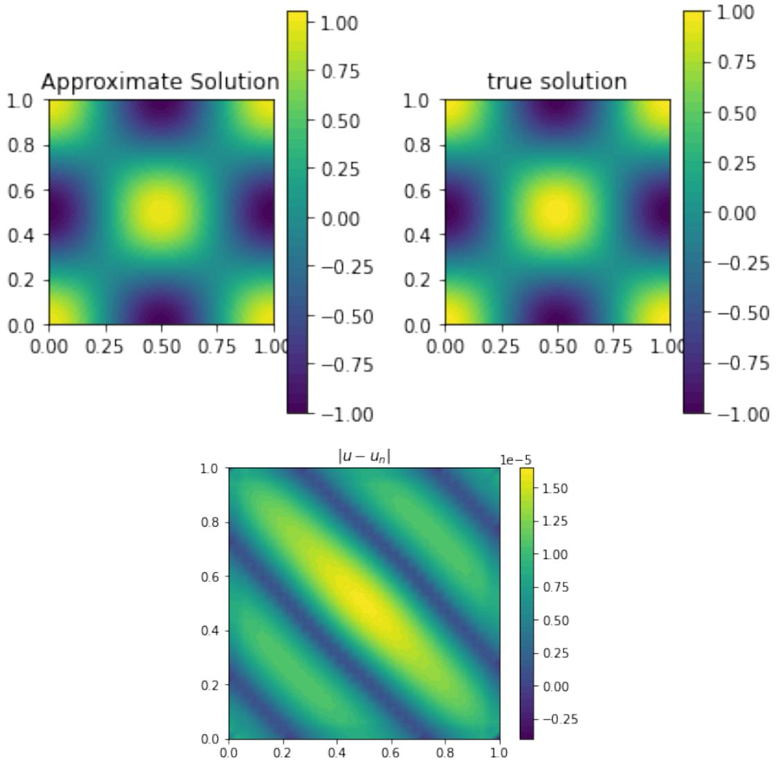
**Figure 2.2** Plot of the true solution  $u(x, y) = \cos(2\pi x) \cos(2\pi y)$  and the approximate FEM solution to the Neumann problem. The third plot is the absolute error between the true solution and the approximate FEM solution.
