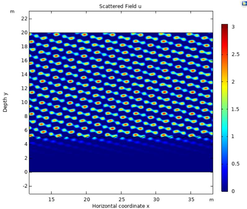
**Figure 2.6** Plot of the Helmholtz solution  $u$  to the water-sediment problem with frequency  $\omega = 2\pi$ . The attenuation  $\alpha = 5$  and we can see damping occurs at the bottom sedimentary layer part. The computational domain is denoted by a parametric curve  $x = s, y = 0.1 \sin(2\pi s) + 5$ .
