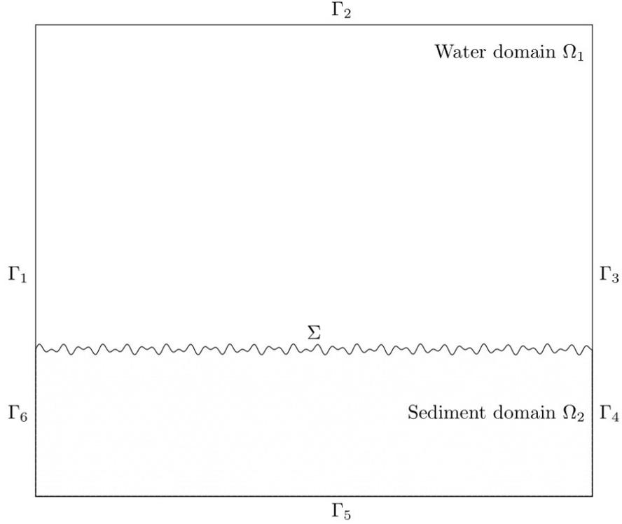
**Figure 3.3** The rectangular two-dimensional non-overlapping partition of the computation domain  $\Omega = \Omega_1 \cup \Omega_2$  for the water-sediment model.  $\Omega_1$  refers to the water domain and  $\Omega_2$  refers to the sediment domain.
