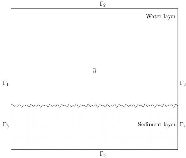
**Figure 2.4** The domain for the water-sediment model. Similar to the domain for the point source Helmholtz problem but with new boundaries created by splitting the left and right sides of the boundary. The boundary conditions include periodic boundary conditions for the top and bottom subdomains.
