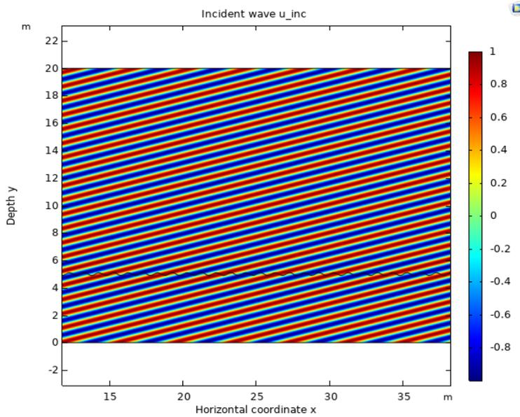
**Figure 2.5** Plot of the incident plane wave  $u_{inc} = \exp\left(i\omega(\cos\theta x + \sin\theta y)\right)$ . The incident angle is  $\theta = 7\pi/12$  and frequency  $\omega = 2\pi$ . The computational domain is denoted by a parametric curve  $x = s, y = 0.1 \sin(2\pi s) + 5$ .
