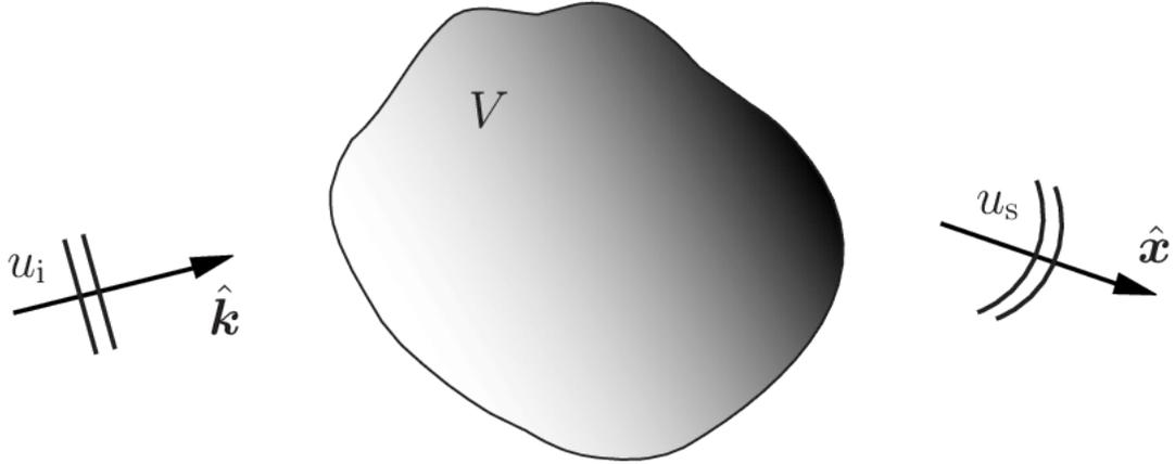
**Figure 1.1** Illustration of a direct scattering problem: The scatterer  $V$  is subject to the incident plane wave  $u_i$  in the  $\hat{\mathbf{k}}$ -direction. Scattering wave  $u_s$  is detected in the  $\hat{\mathbf{x}}$ -direction, adopted from (Sohl et al., 2008).
