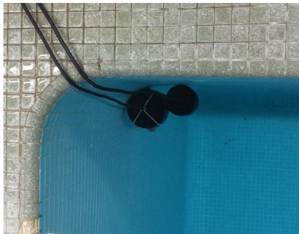
Figure 3.1 Vector transmitter of the MISO system includes a ring transducer (left) with four segments which acts as two orthogonal dipoles for two independent data streams, plus a nearly co-located scalar transducer (right) for the third data stream. The transducers are at the same depth and there is no spacing between them.
