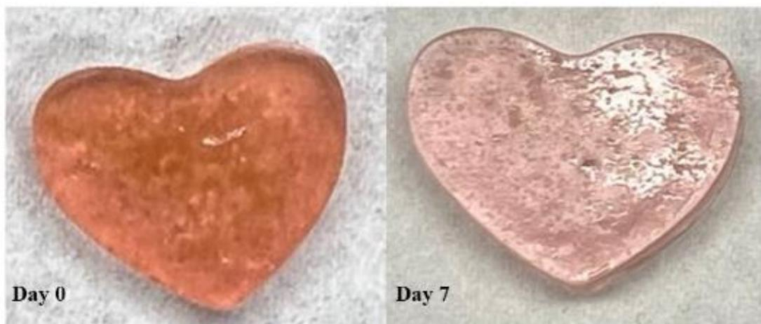
**Figure 3.9** Films preparation steps include mixing the PETMP, TMPTMA and BD-I-TMG (ratio: 1 mmol : 1 mmol : 0.05 mmol) in a glass vial, loading the mixtures in the mold, then the mixture was irradiated by the Thorlab's M505L3 LED light source (nominal wavelength 505 nm, power density is 80 mW/cm<sup>2</sup>, irradiated distance: 1 cm) for 30 min. After solidifying, the film was soaked in DMSO for 7 days.
