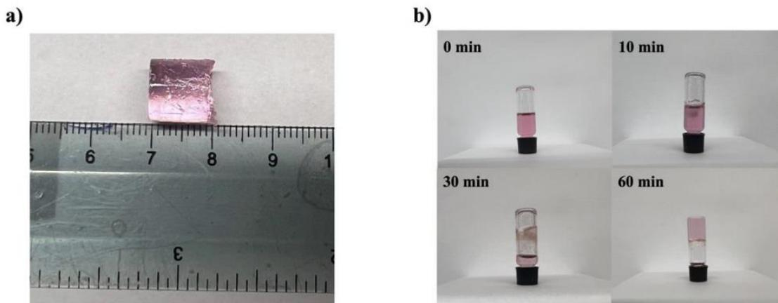
**Figure 3.10** a) Green light-initiated polymer at the thickness of 10 mm. b) Photos of experiments demonstrating the photocuring conditions over different light irradiation time. The polymer networks formed through the monomer cross-linking PETMP/TMPTMA (molar ratio = 1:1) and 2.5 mol % BD-I-TMG loading. The sample was irradiated with 80 mW/cm<sup>2</sup>, 505 nm LED light for up to 60 min without dark cure. The irradiated distance is 1 cm.
