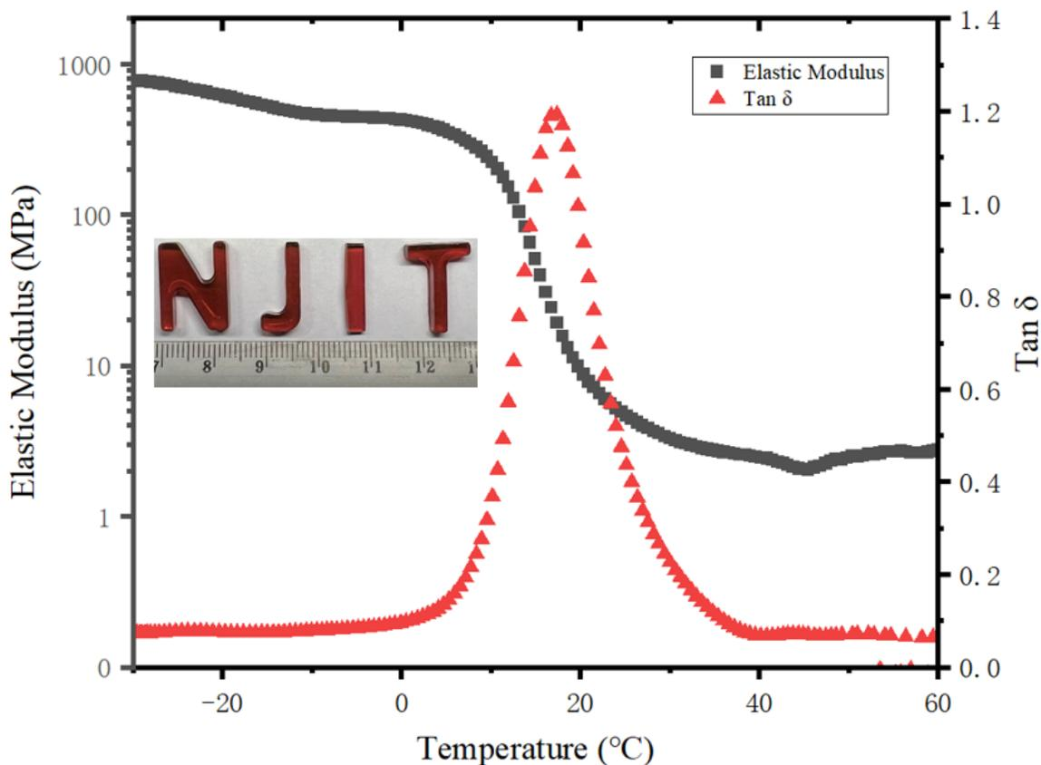
**Figure 3.5** Plots of  $\tan \delta$  and elastic modulus vs temperature for polymer networks formed through the monomer cross-linking PETMP/ TMPTMA (molar ratio = 1:1) and 2.5 mol % BD-I-TMG catalyst loading. The sample was irradiated with  $80 \text{ mW/cm}^2$ , 505 nm LED light for 1 h. The irradiated distance is 1 cm.
