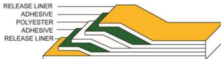
Figure 5.1 Cross-section of layers of adhesive tape.
