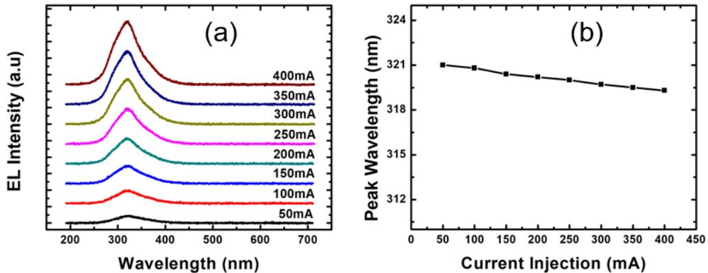
**Figure 6.11** (a) Electroluminescence Spectra of GaN/AlGa<sub>N</sub> Based UV-B Nanowire LED from 50 mA to 450 mA (b) Variation of Peak Wavelength with Current Injection.
