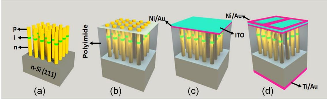
**Figure 2.8** Schematic diagram of fabricated nanowire LED.
