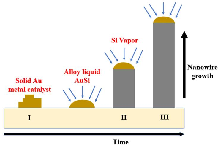
**Figure 2.1** VLS growth process depiction: I) semiconductor in vapor phase is introduced into the system with metal catalyst on the substrate surface, II) the formation of liquid droplets on the substrate surface near or above the eutectic temperature, and III) supersaturation and the formation of nucleation sites and the nanowire axial growth.
