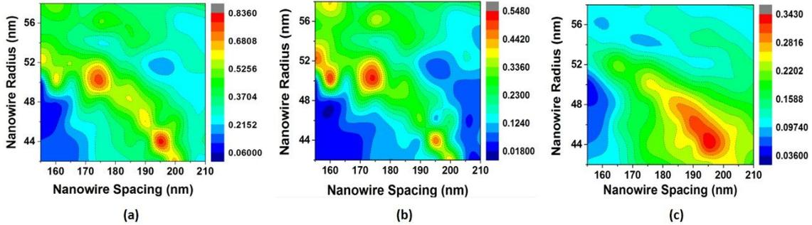
**Figure 6.5** The contour plots show light extraction efficiencies with the radius ranges of 42 – 58 nm, and spacing ranges of 155 – 210 nm for (a) the structure without material absorption, (b) light power loss due to material absorption, (c) the structure with material absorption.
