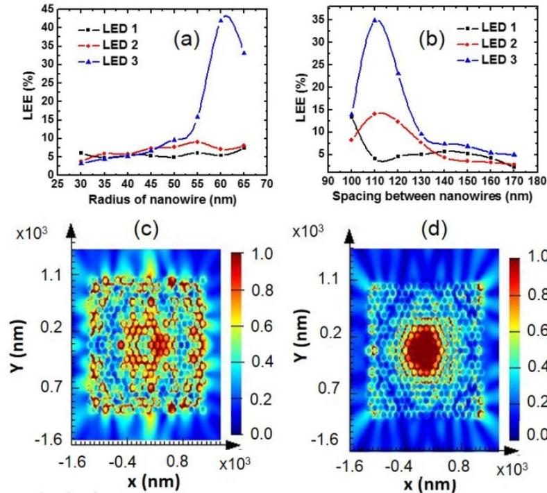
**Figure 5.2** (a) Variation of LEE with change in spacing (for a constant radius of 50 nm) and (b) change in radius (constant spacing of 130 nm). (c) electric field distribution plot from top monitor for a flip-chip on metal. (d) electric field plot from top monitor for a normal p-i-n LED structure on Si substrate.
