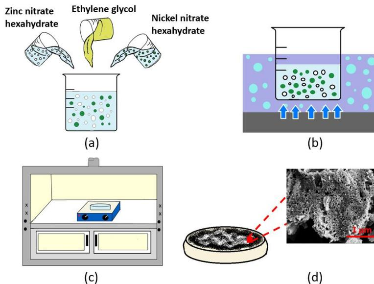
**Figure 8.1** Schematic of Polyol Fabrication Route of Ni-ZnO Structure with (a) Mixing of Precursors Including Zinc Nitrate Hexahydrate, Nickel Nitrate Hexahydrate and Ethylene Glycol. (b) Sonication of the Reagent Mixture for 15 minutes. (c) Burning of the reagent Mixture at 250<sup>0</sup> C on a Hot Plate kept in Fume Hood and (d) Formation of Highly Porous Ni-ZnO Composite with Inset Depicting SEM of same.
