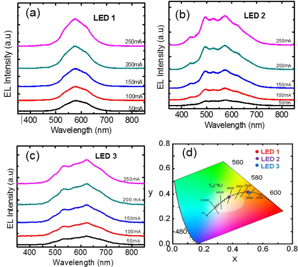
**Figure 3.6** EL Spectra of three distinct LEDs (a) LED 1 (b) LED 2 (c) LED 3. (d) CIE 1931 chromaticity diagram illustrating the emission characteristics of three different InGaN/AlGaIn nanowire LEDs.
