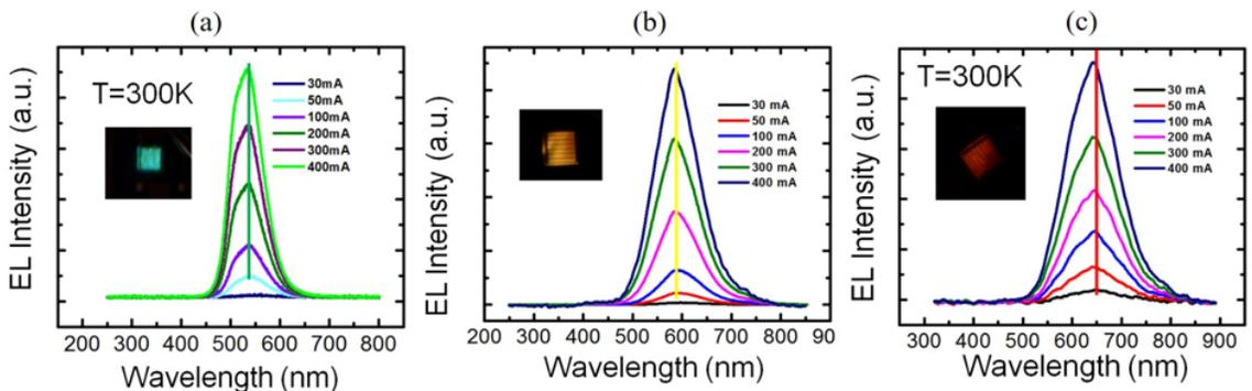
**Figure 3.2** Room temperature electroluminescence spectra under different injection currents for (a) green, (b) yellow, (c) red nanowire LEDs. The inset of each figure shows the corresponding light emissions from green, yellow and red nanowire LEDs.
