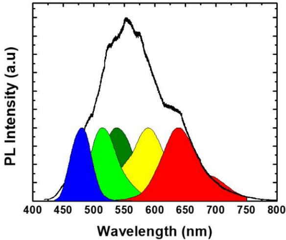
**Figure 4.2** Photoluminescence spectra depicting phosphor free white LED with GaN/InGaN nanowire system with normalized individual color spectra shown inside.
