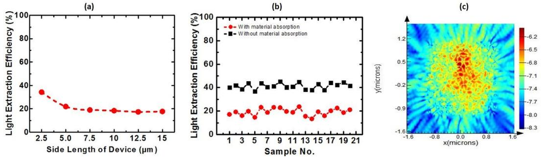
**Figure 6.7** (a) Dependence of the light extraction efficiency on the various device sizes, (b) the light extraction efficiency for 20 different structures with random nanowire spacing and random nanowire radius, (c) the simulated mode profiles with the random nanowire spacing and radius.
