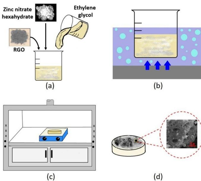
**Figure 7.1** Schematic of polyol fabrication route of ZnO structure with (a) mixing of precursors including zinc nitrate hexahydrate, ethylene glycol and RGO (b) sonication of the reagent mixture for 15 minutes (c) burning of the reagent mixture at 250°C on a hot plate kept in fume hood and (d) formation of highly porous ZnO-G composite with inset depicting SEM of same.
