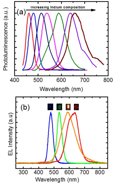
**Figure 3.3** (a) Normalized room temperature photoluminescence spectra of multiple emission colors from multiple InGaN/AlGaN nanowire LEDs. (b) electroluminescence spectra of various InGaN/AlGaN LEDs with distinct emission colors, along with their optical image.
