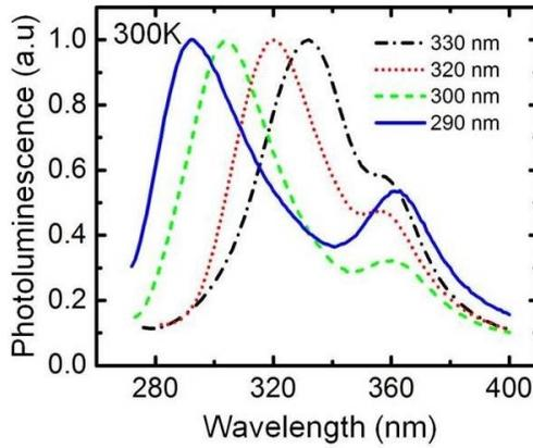
**Figure 6.10** Normalized room temperature photoluminescence spectra of UV-B lights at 290 nm, 300 nm, 320 nm and 330 nm from multiple AlGa<sub>N</sub> nanowire LEDs.
