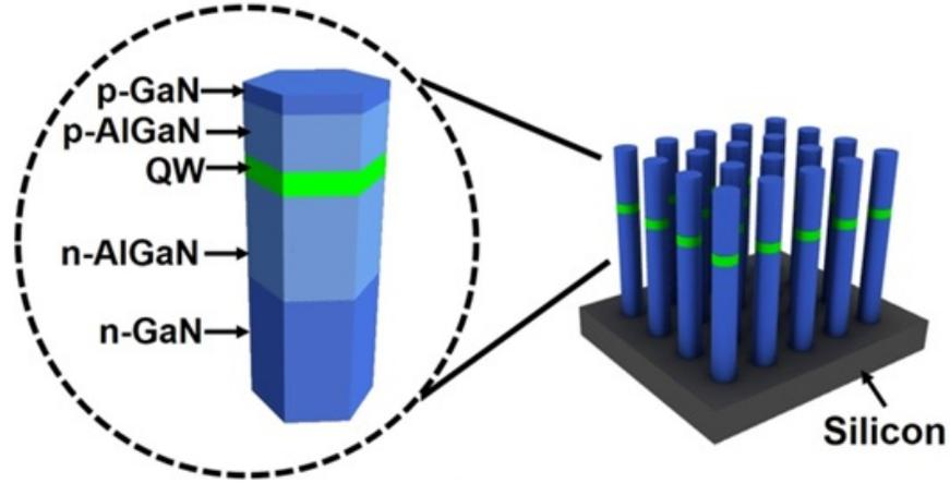
**Figure 6.2** Schematic illustration of GaN based nanowire UV-B LED structure with inset image presenting the detailed structure of n-AlGaN layer, a quantum well active region, a p-AlGaN layer, and p-GaN layers.
