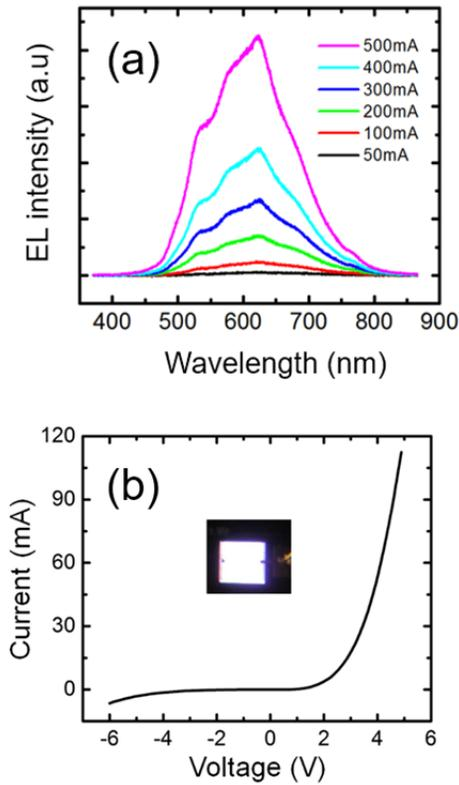
**Figure 3.4** (a) Room temperature electroluminescence spectra of an InGaN/AlGaN core-shell LED under different injection current levels (b) current-voltage characteristics of the core-shell nanowire LED along with the optical image of the white LED.
