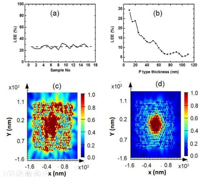
**Figure 5.3** (a) LEE for 16 different random structures with multiple nanowire diameter and nanowire spacing and between them. (b) variation of p-type height with LEE of a flip chip (n-i-p) structure on metal. (c) and (d) electric field contour plots for a typical random flip chip structure on metal and a random normal (p-i-n) structure on Si Substrate.
