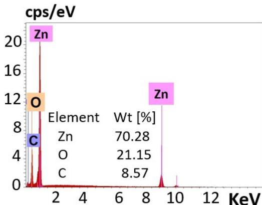
**Figure 7.5** Elemental EDS analysis for ZnO-G sample.
