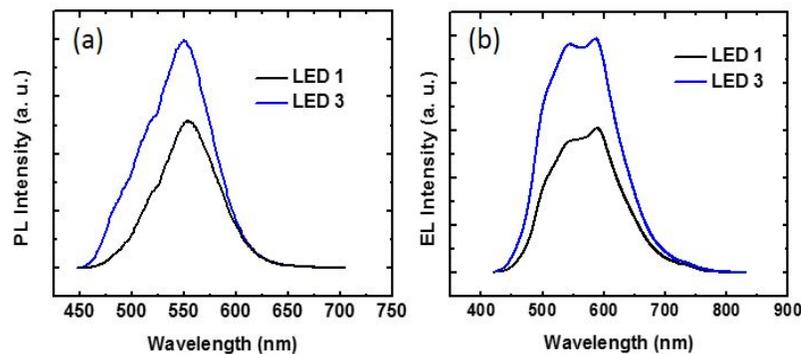
**Figure 5.6** Room Temperature (a) photoluminescence spectra of flip-chip nanowire LED on Cu (blue curves) and conventional nanowire LED on SOI substrates (black curves). (b) electroluminescence spectra of flip-chip nanowire LED on Cu (blue curves) and conventional nanowire LED on Si substrates (black curves).
