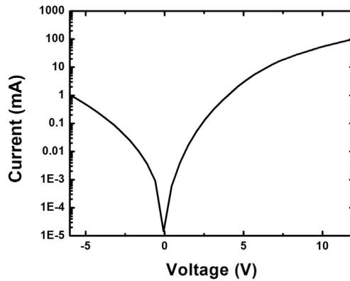
**Figure 6.12** Current–Voltage Characteristics of the AlGaIn Nanowire LED.
