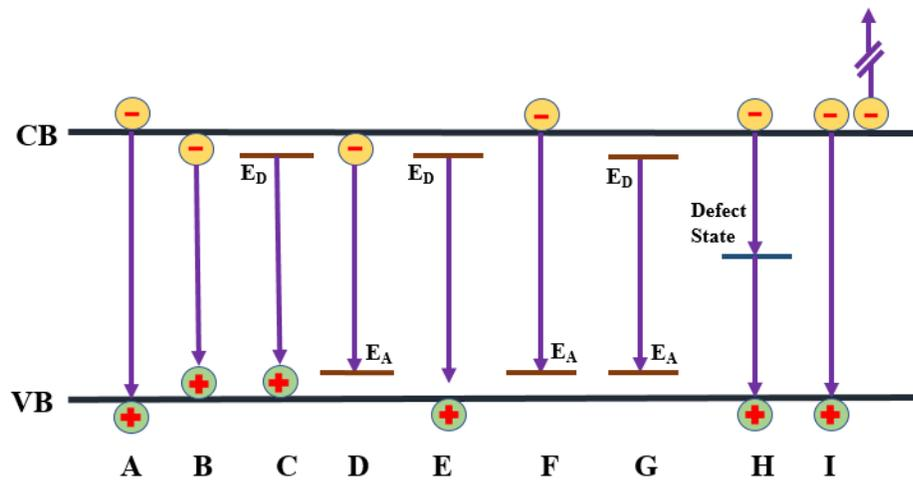
**Figure 2.9** Radiative and non-radiative optical transitions. radiative transitions include A (band to band), B (free exciton), C and D (bound excitons), E (donor to valence band), F (conduction band to acceptor band), G (donor to acceptor pair) while non-radiative transitions include H (defect state related) and I (auger recombination).
