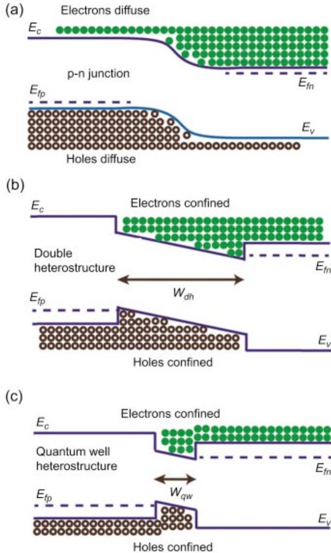
**Figure 1.5** Conduction band diagrams illustrating confinement and carrier diffusion in (a) a typical *p-n* junction, (b) a double heterostructure (heterojunction), and (c) QW heterostructure. As  $W_{qw} < W_{dh}$ , the carrier confinement is pronounced in a QW as compared to that of a double heterostructure leading to a higher carrier concentration in QW.
