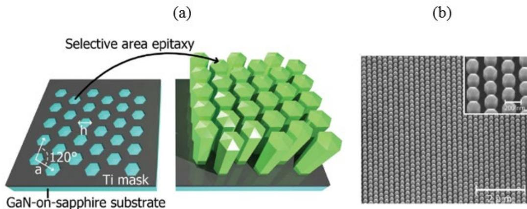
**Figure 2.3** (a) Nanoscale arrays developed by e-beam lithography process on a Ti mask on planar GaN template on c -plane sapphire substrate. (b) SEM image showing GaN nanowire arrays selectively grown in the opening apertures.
