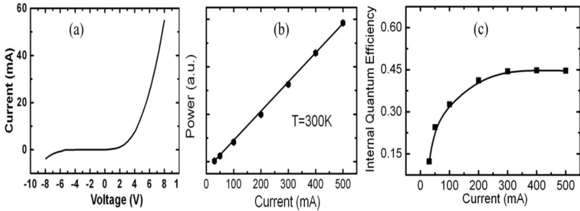
**Figure 3.7** (a) Room temperature current-voltage characteristic of the yellow nanowire LED. (b) light-current characteristic of yellow nanowire LED under different injection currents. (c) room temperature internal quantum efficiencies of typical yellow LED versus various current levels.
