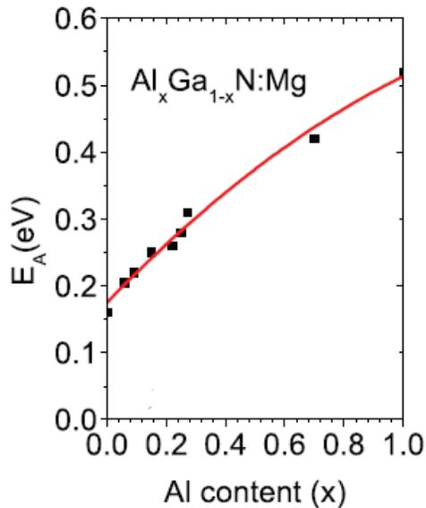
**Figure 6.1** Mg acceptor activation energy level in AlGa<sub>x</sub>N as a Function of Al composition for Al<sub>x</sub>Ga<sub>1-x</sub>N alloys [240].
