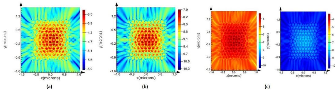
**Figure 6.6** The simulated mode profiles with the optimized nanowire parameters for the spacing  $\sim 195$  nm and radius of the nanowires  $\sim 44$  nm for the UV LED (a) without and (b) with material absorption, (c) the simulated mode profiles with same intensity scale.
