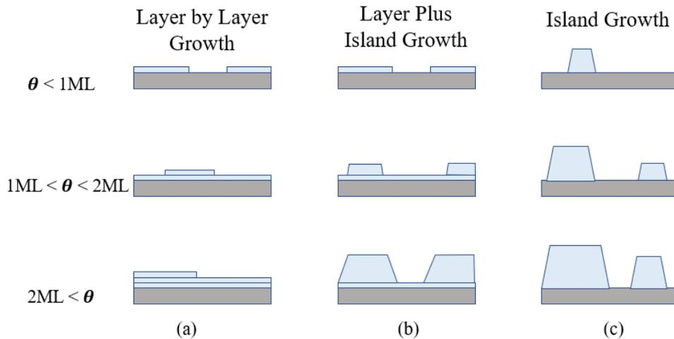
**Figure 2.6** Schematic representation of different growth modes for film formation in MBE for multiple coverage ( $\theta$ ) regimes (ML refers to monolayer) (a) layer by layer or Frank-von der Merwe mode (b) Layer plus island growth or Stranski -Krastranov growth mode and (c) Island growth or Vollmer-Weber growth mode.
