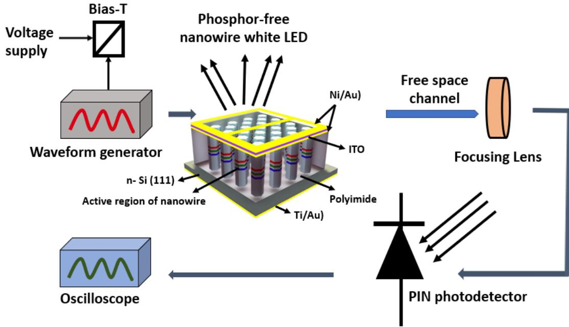
**Figure 4.5** Schematic of the Experimental Setup for VLC.
