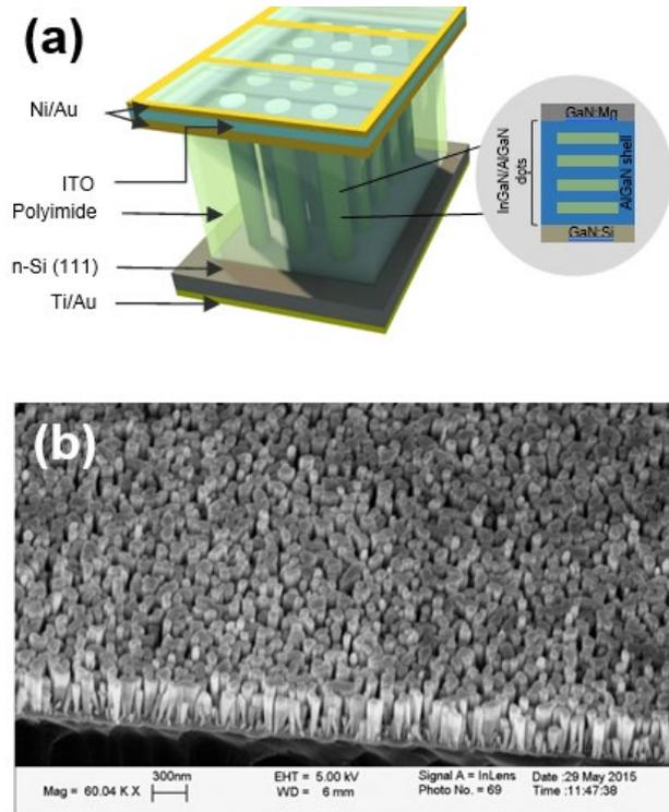
**Figure 3.1** (a) Schematic illustration of an InGaN/AlGaN dot-in-a-wire core-shell LED heterostructure on Si substrate. Inset depicts the layer by layer structure. (b) A 45° tilted SEM image of a typical InGaN/AlGaN core-shell nanowire LED sample.
