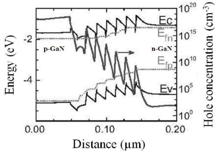
**Figure 1.11** Simulated band diagrams and hole concentrations for LEDs with InGaN/GaN MQW LEDs under +6 V forward bias at 300 K. Hole distributions within the QWs are shown by thick solid lines while dashed lines represent quasi-fermi levels. Source: [93].
