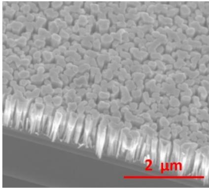
**Figure 4.1** 45<sup>0</sup> tilted scanning electron microscopy image illustrating the surface morphology of the molecular beam epitaxy grown InGaN/AlGaN dot-in-a-wire heterostructures grown on a *n*-type Si (111) substrate.
