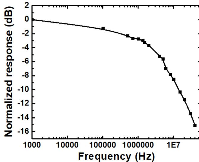
**Figure 4.7** Frequency response of phosphor-free nanowire white LED.
