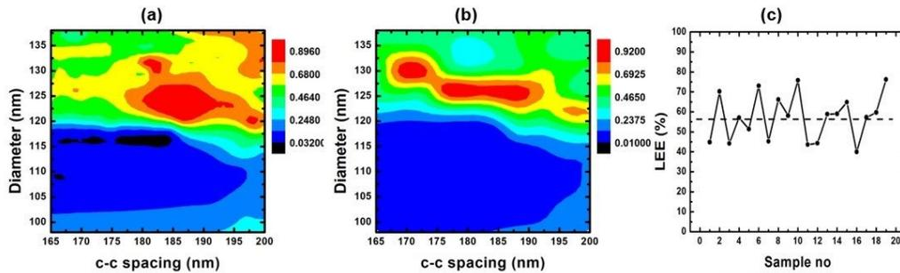
**Figure 6.3** The contour plots for AlGaN based nanowire UV-B emitters depicting LEEs with the radius ranges of 49–69 nm, and center to center (c-c) spacing ranges of 165–200 nm with light sources of (a) 290 nm (b) 320 nm and (c) LEE for 19 different random structures with different nanowire diameter and nanowire spacing between them for a light source of 290 nm.
