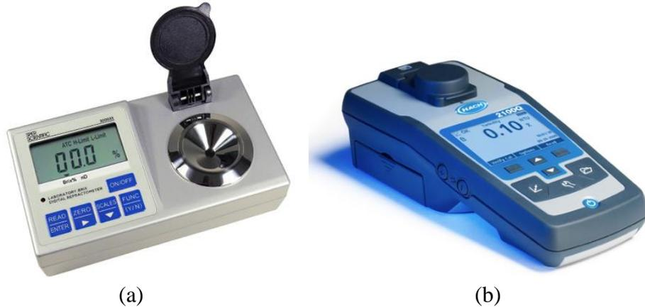
**Figure 2.2** Portable equipment used in this work: (a) Sper Scientific Laboratory 300033 refractometer and (b) Hach-2100Q turbidimeter.
