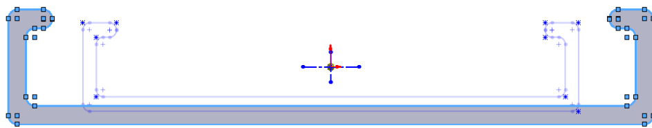
Figure 3.5 Scaling the profile to adjust for drawdown effect.
