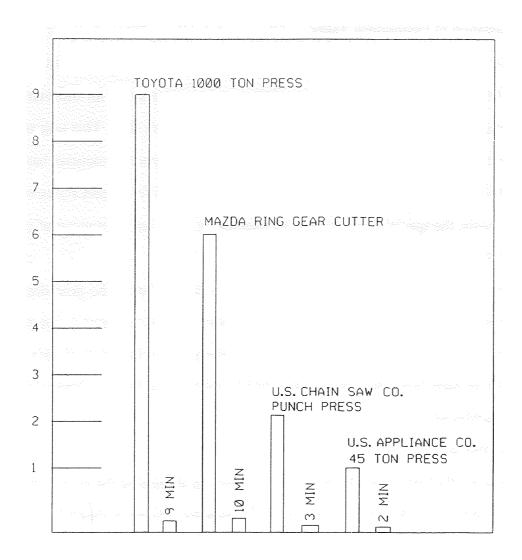
FIGURE 8. EXAMPLES OF SETUP TIME REDUCTION
