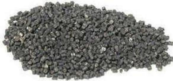
**Figure 3.1** NdFeB Bonded Composites Granules used for the experiment.
