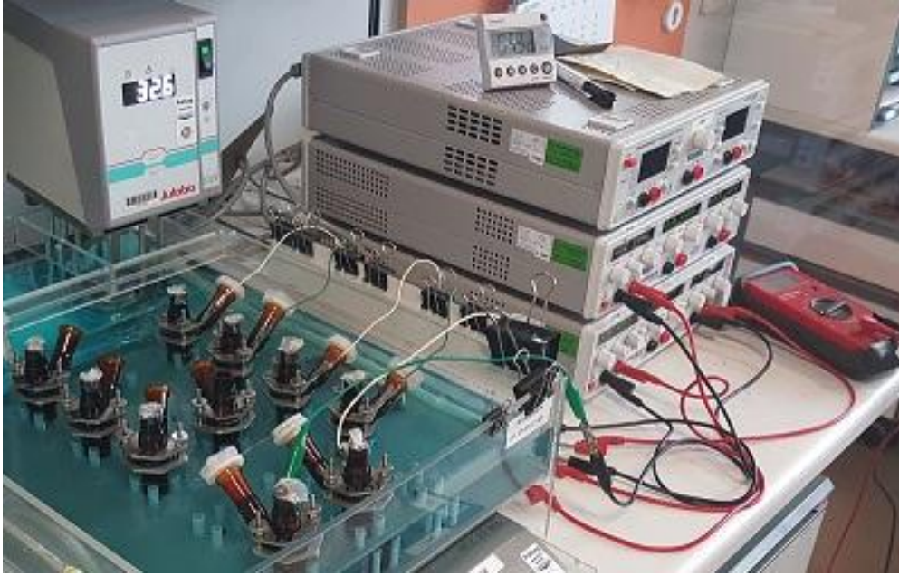
Figure 2.5 Two-chamber franz cell system with electrical current.
