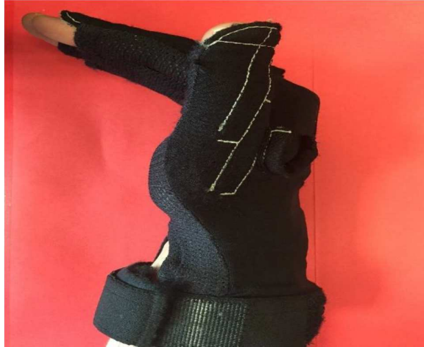
Figure 6.1 Cyber Glove was worn by patients to acquire their kinematic data during the finger extension movements and deliver PAS stimulation to the affected hand. PAS was triggered by a change in the angle of five degrees from the patient's relaxed position following the presentation of a move cue on the screen.
