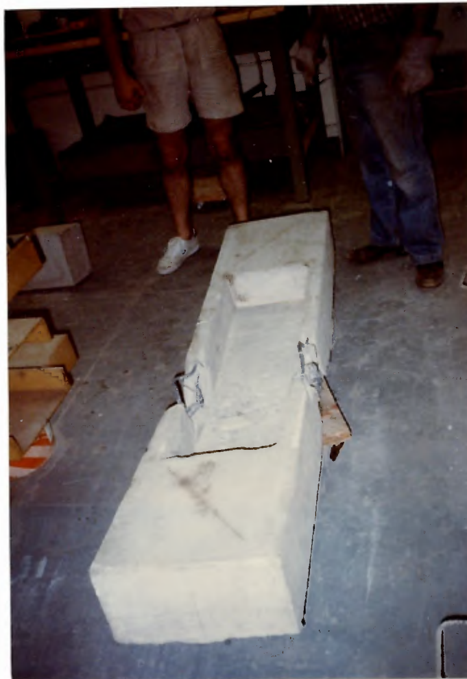
Fig. 3.4. Column after compression failure.
