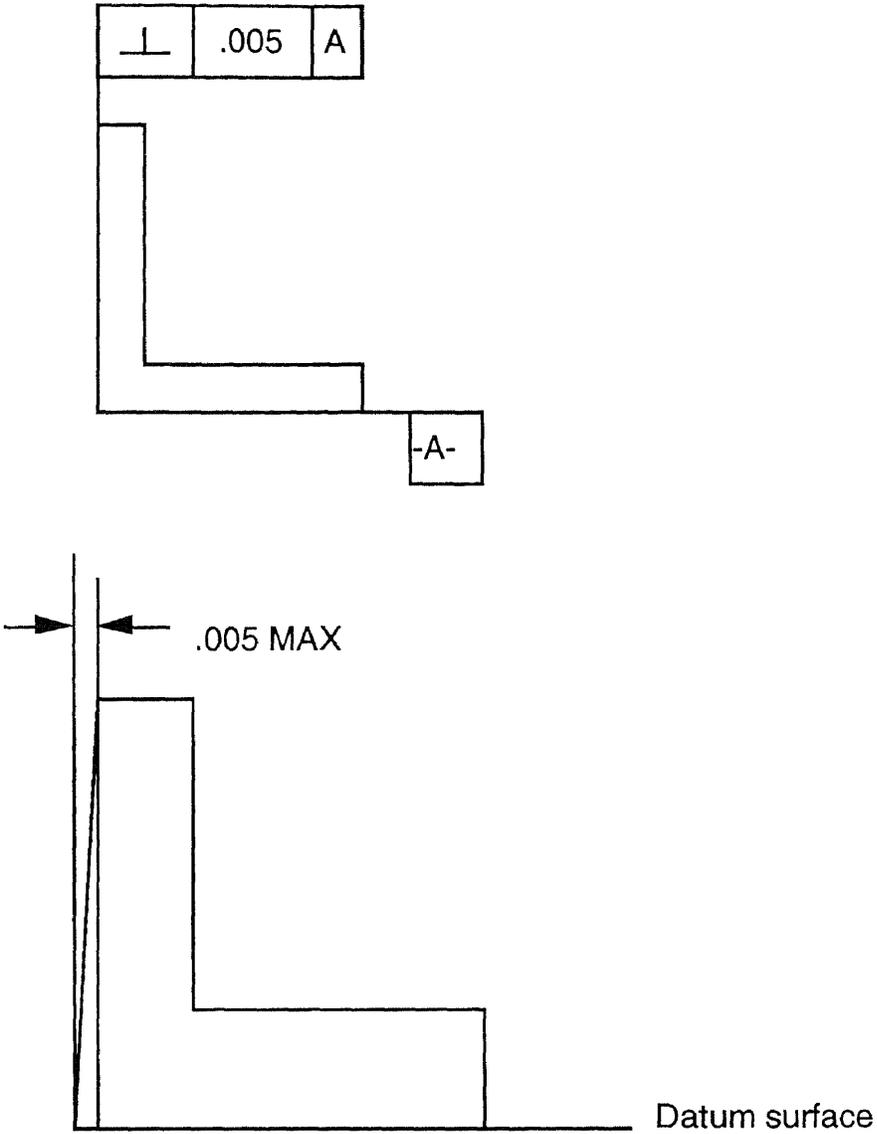
Figure 17 Perpendicularity
