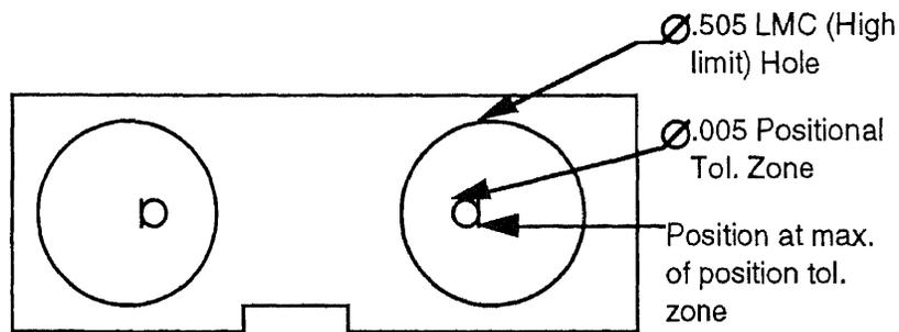
Figure 22 LMC When High Limit
