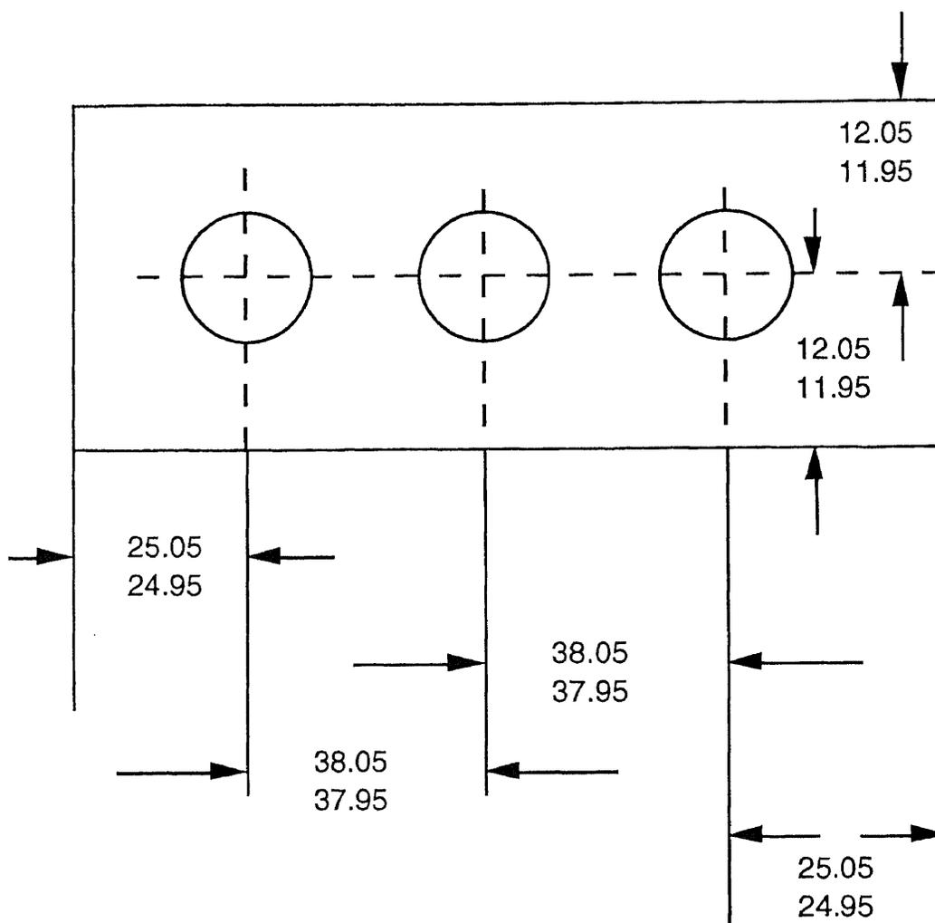
**Figure 12** Accumulation of tolerance
