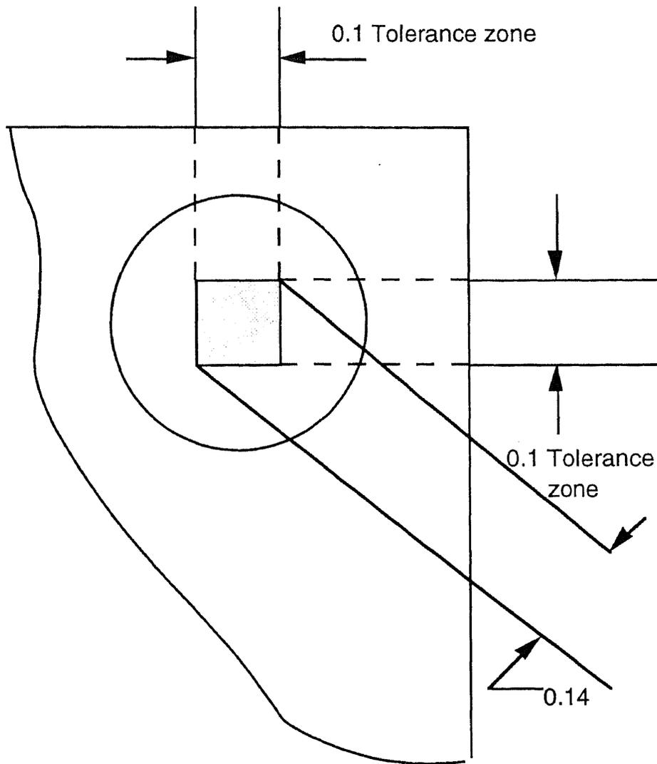
**Figure15** Size Tolerance
