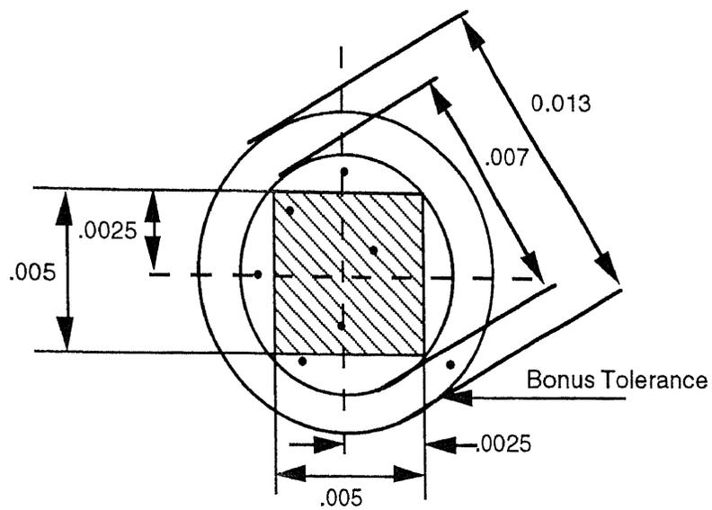
**Figure 24** Concept of Bonus Tolerance
