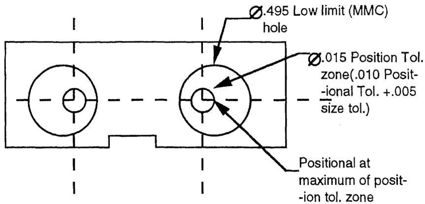
Figure 23 LMC When Low Limit
