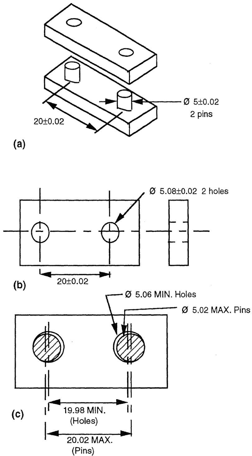
Figure 20 (a), (b), (c) Maximum Material Condition
