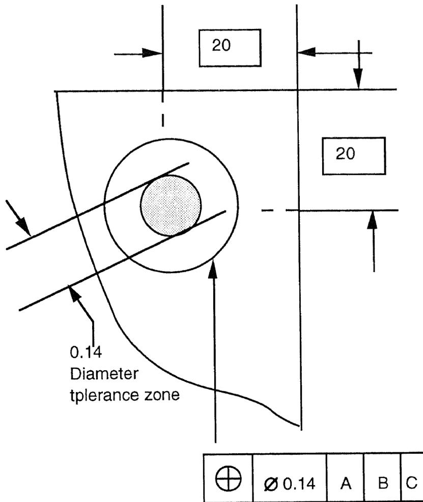
**Figure 16** Positional tolerancing
