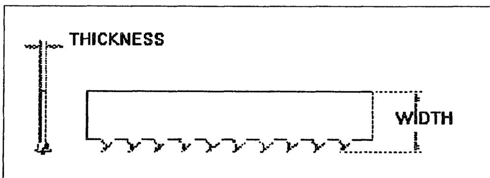
Figure 3 Band-Saw Blade
