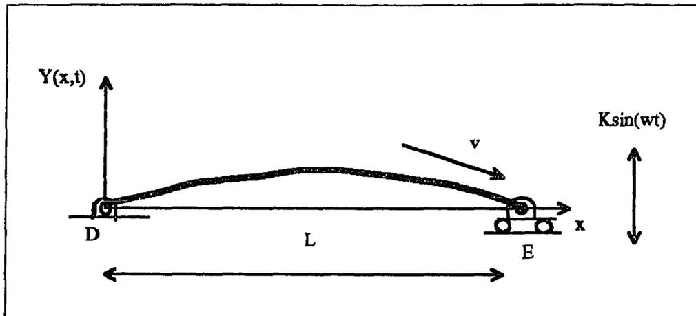
Figure 4 The Axially Moving Bernoulli-Euler Beam Under Tension
