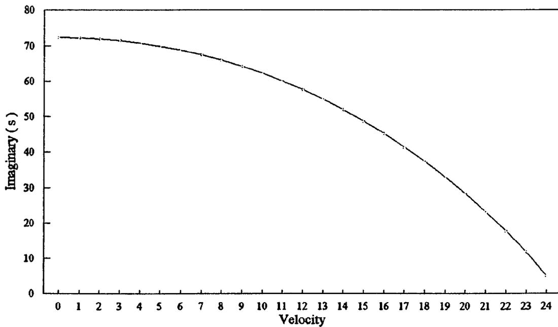
**Figure 22** Imaginary part of the Eigenvalue versus Velocity at Tension=575
