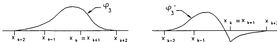
Fig. 3-3 Cubic B-spline and Its First Derivative ( C^1 at knot x_k = x_{k+1} and C^2 elsewhere)
