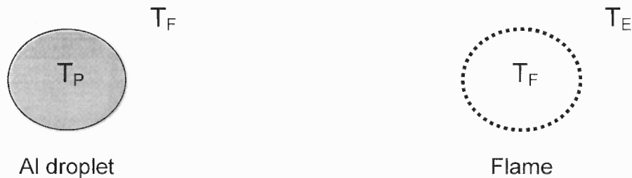
Figure 5.9 To calculate heat transfer from flame to particle the particle is assumed to be surrounded by hot gas at the flame temperature T_F (left sketch). To calculate heat loss from flame to environment, the flame is assumed to sit directly on the particle surface and lose heat to the environment temperature T_E (right sketch).
