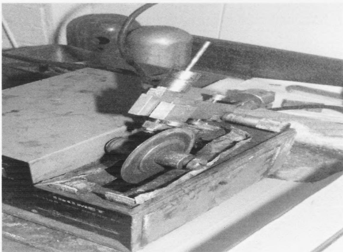
**Fig. 4.18** Schematic of a Cutting Wheel
