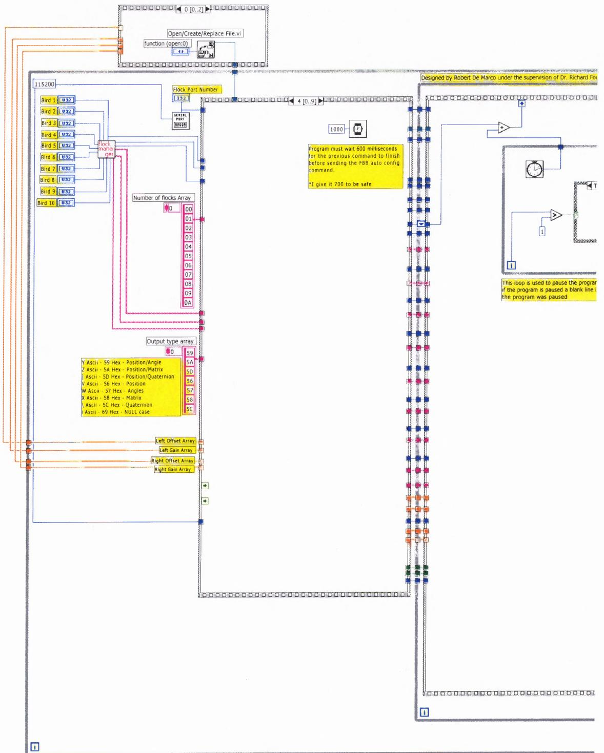
Figure A.5 Fifth stage in initialization is a delay of one second to allow the FBB auto configuration command time to start.
