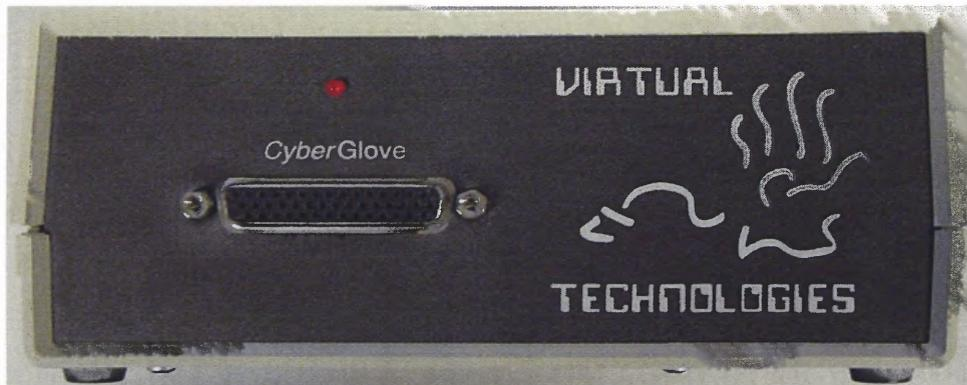
**Figure 2.13** The Cyberglove Interface Unit (CGIU).
