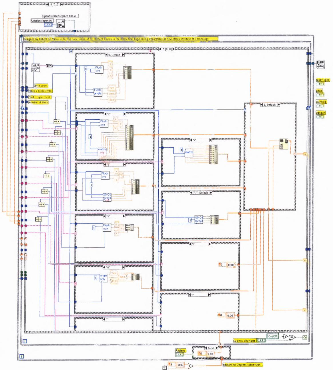
**Figure A.17** Seventh stage in data acquisition converts hexadecimal Cyberglove and FOB data into the desired output type.
