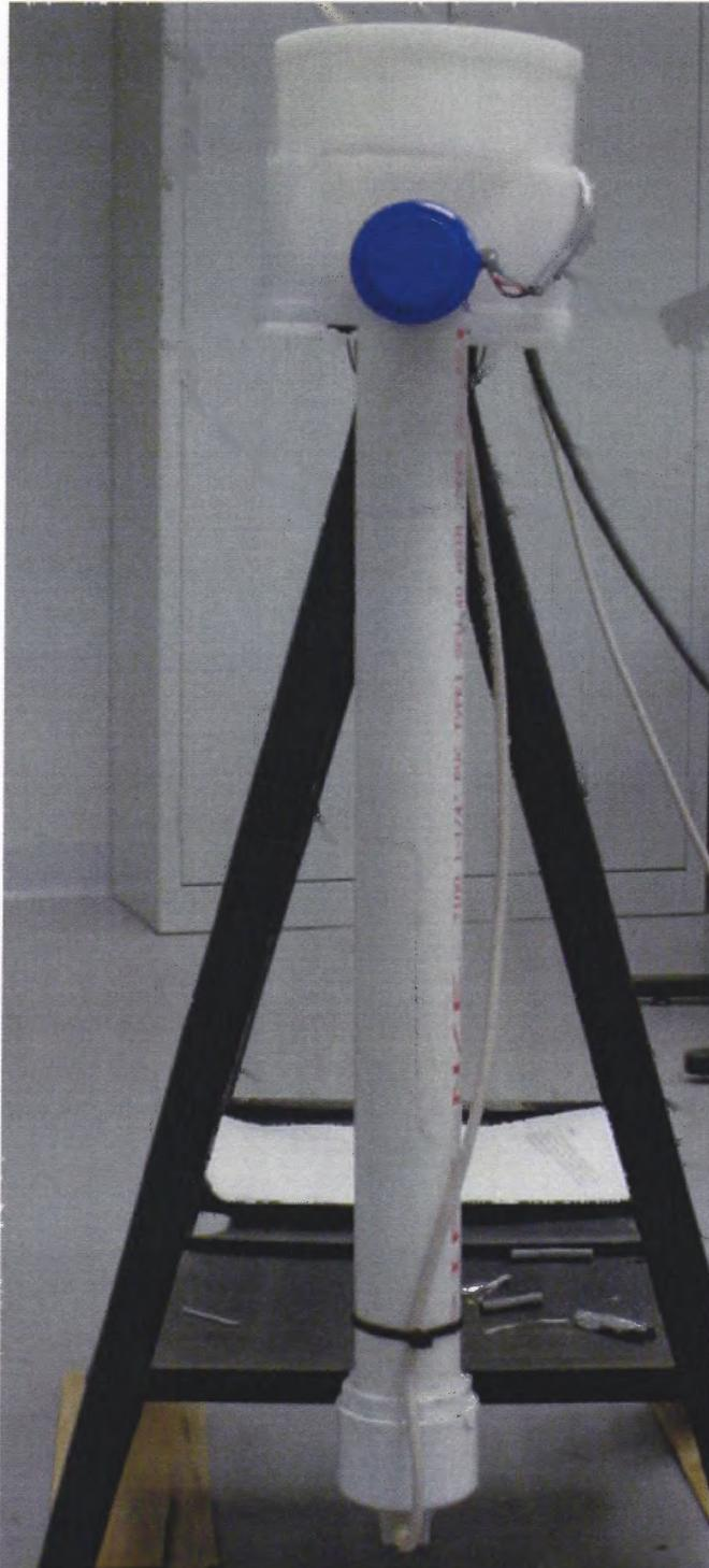
**Figure 3.5** Pendulum calibration setup with potentiometer and FOB.
