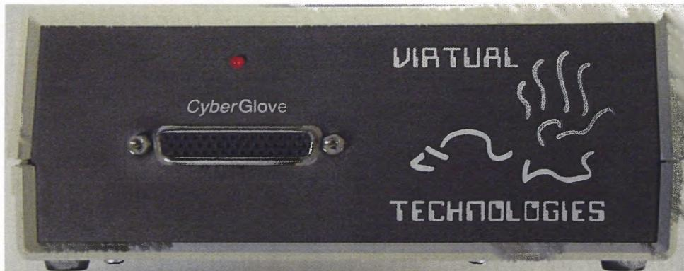
**Figure 2.13** The Cyberglove Interface Unit (CGIU).
