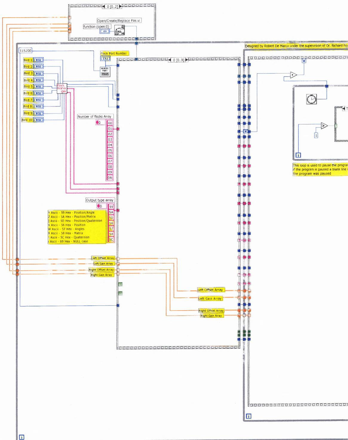
**Figure A.2** Second stage in initialization writes a header file to the ASCII file to be recorded.
