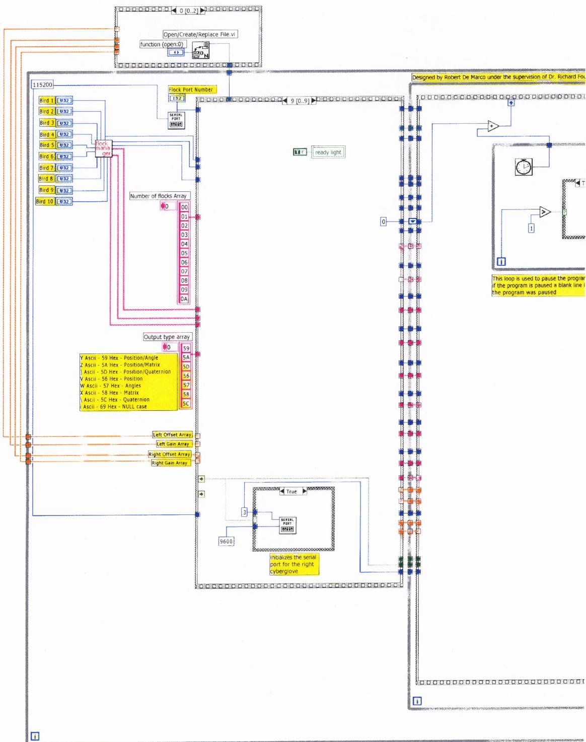
**Figure A.10** Last stage in initialization, is used to turn on ready light and initialize the serial port for the right Cyberglove.
