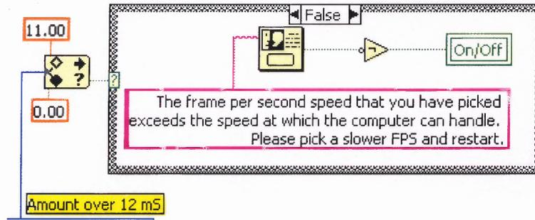
**Figure 4.25** A part of dynamic timing that produces error if the frame rate is exceeded.
