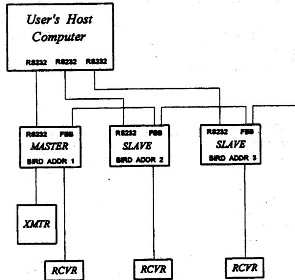
**Figure 2.6** Flock of Birds configured for multiple sensors by giving each sensor its own dedicated serial connection to the computer. The XMTR is the transmitter and the RCVR is the sensor (Ascension Technology Corporation, 1999).
