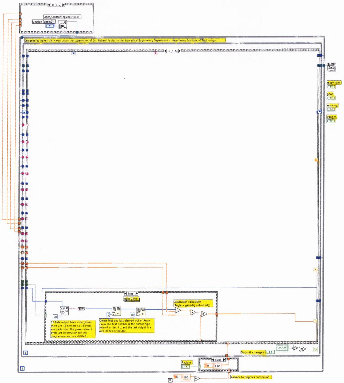
Figure A.16 Sixth stage in data acquisition reads data from the right Cyberglove.
