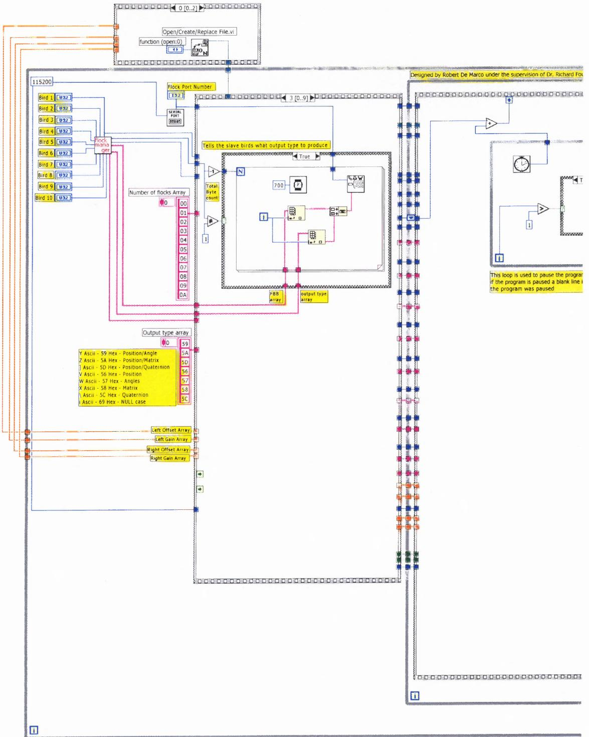
Figure A.4 Fourth stage in initialization sets the output type for active slave birds.
