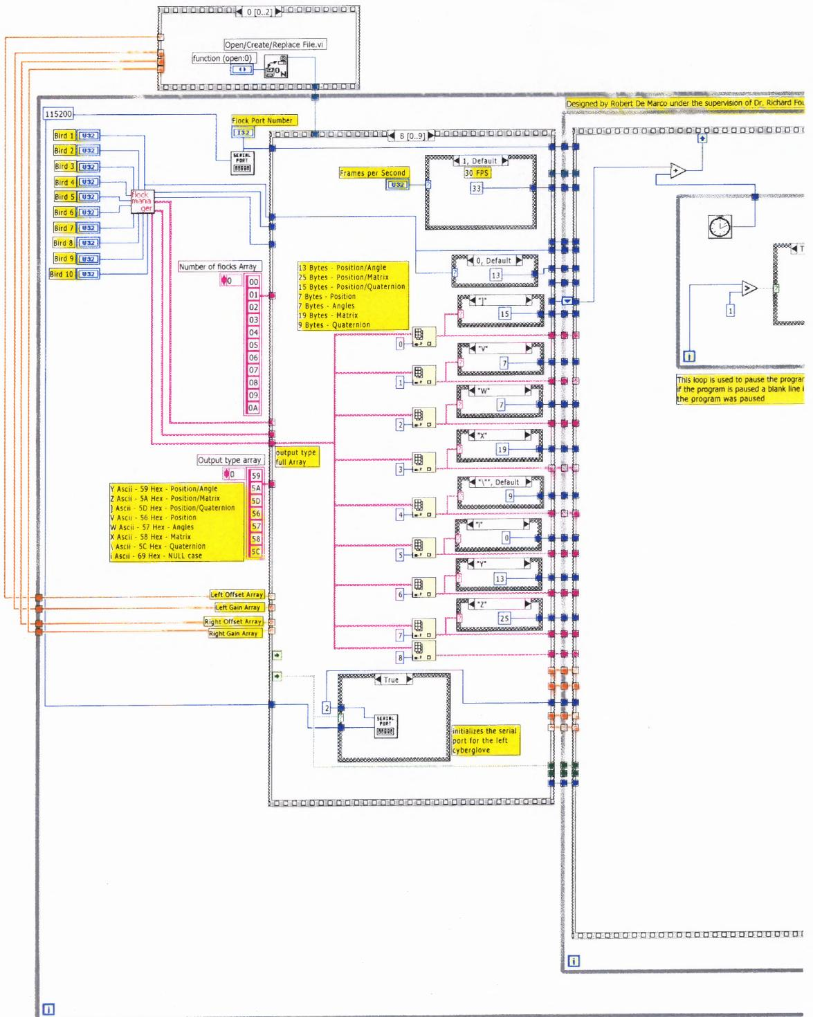
Figure A.9 Ninth stage in initialization is used to initialize the serial port for the left Cyberglove and to pass the byte count for each sensor into main loop.
