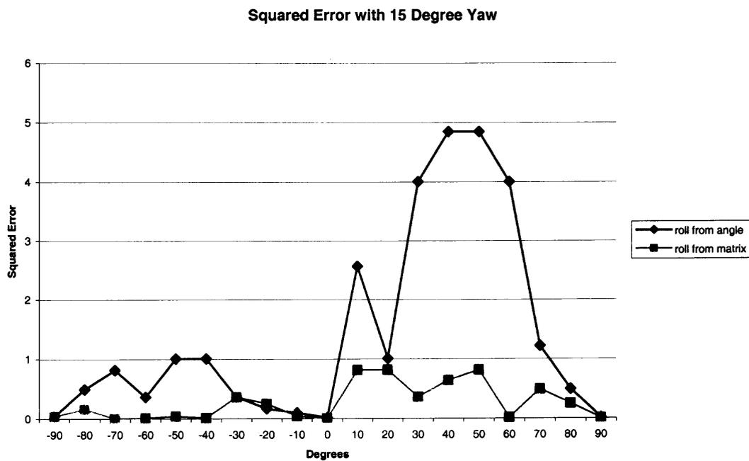
**Figure 3.7** Plot of squared error at 15-degree yaw showing how the squared error differs for different output types. The roll from angle starts to increase while roll from matrix remains semi-linear.
