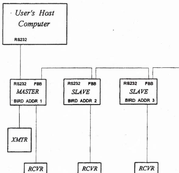
**Figure 2.7** Flock of Birds configured for multiple sensors by using the master slave configuration, which utilized the FBB. For each bird, the XMTR is the transmitter and the RCVR is the sensor (Ascension Technology Corporation, 1999).
