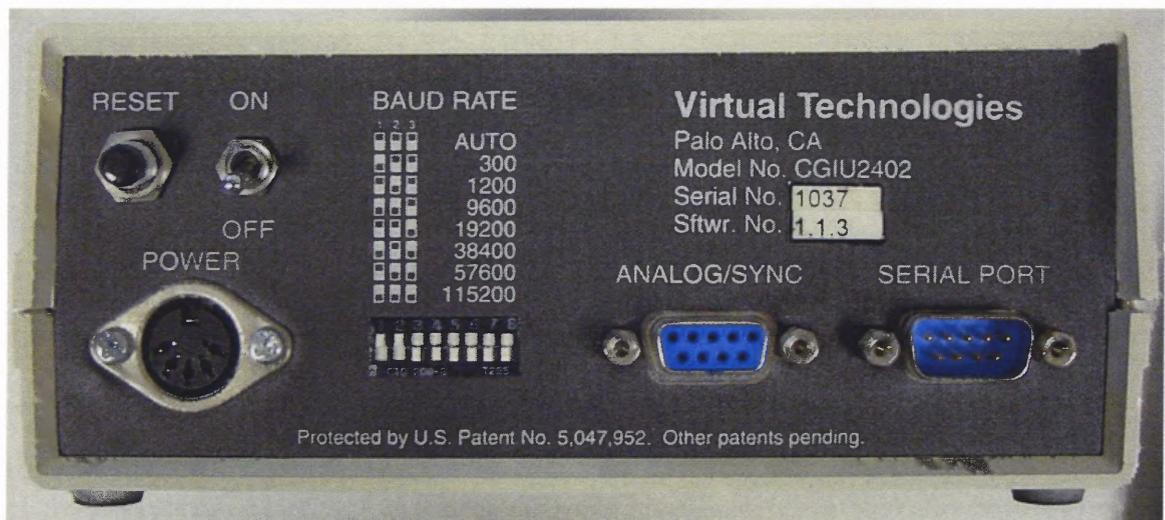
**Figure 2.15** Back of the Cyberglove Interface Unit
