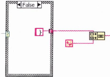
**Figure 4.32** The last stage of the sequence show how the '}' is written and concatenated with a line return.
