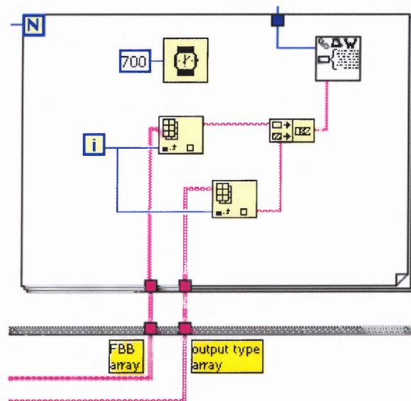
**Figure 4.10** A portion of the VI Cyber Flock showing how all slaves are initialized.
