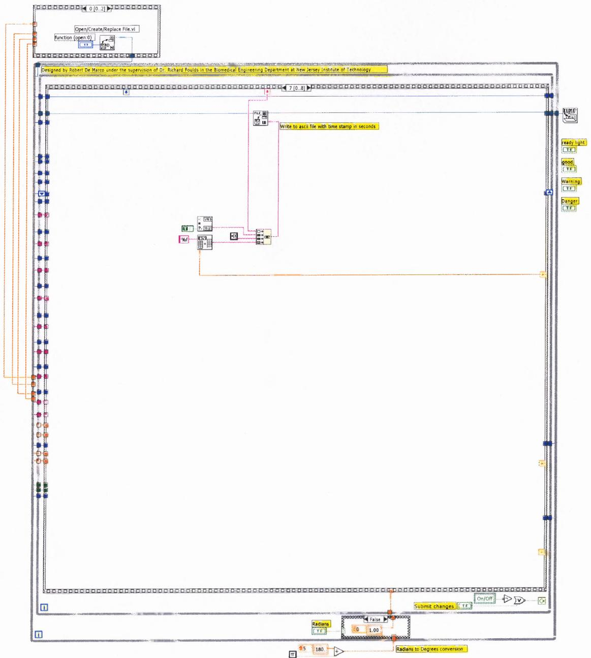
**Figure A.18** Eighth stage in data acquisition writes Cyberglove and FOB data to an ASCII file.
