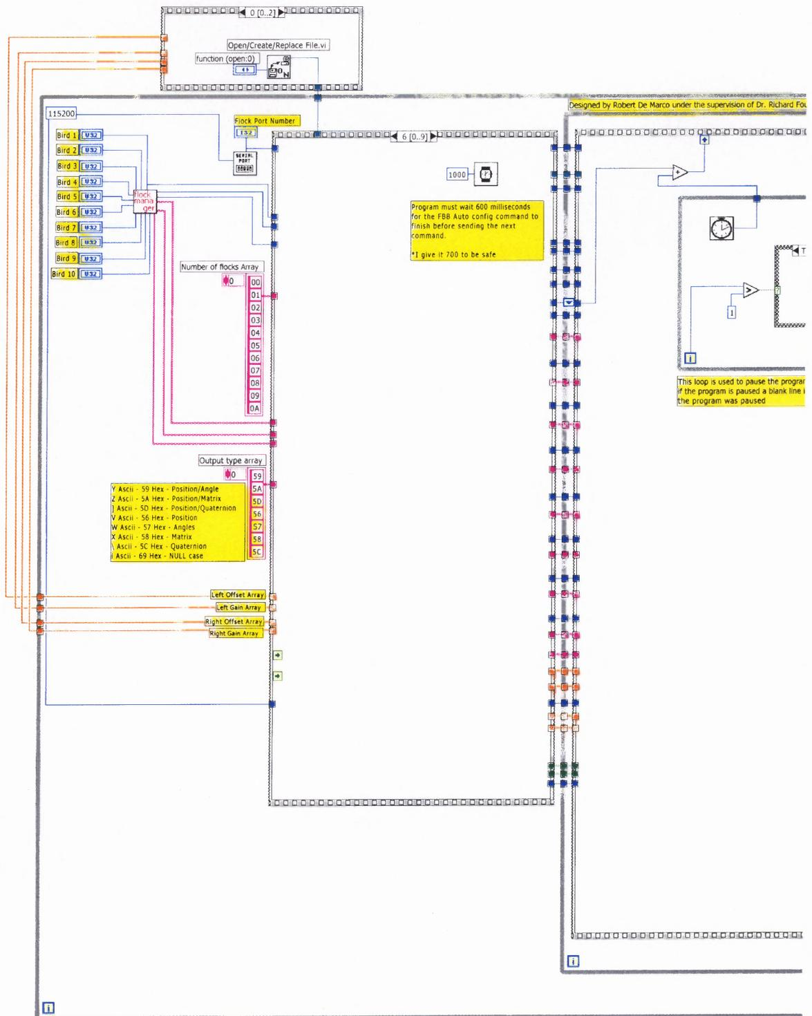
**Figure A.7** Seventh stage in initialization is a delay of one second to allow the FBB auto configuration command time to finish.
