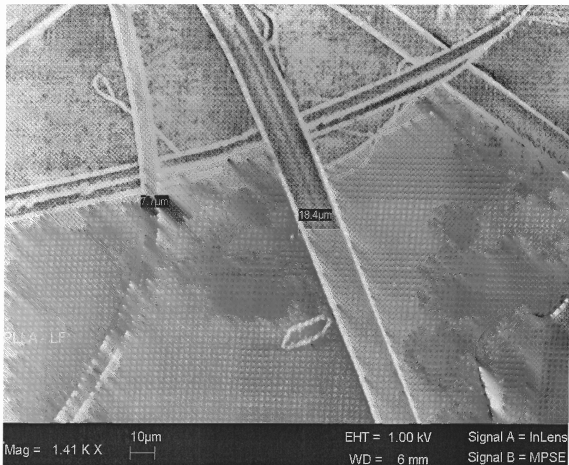
Figure 5.1 SEM image of PLLA-LF (18.4 μm).
