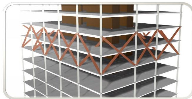
Outrigger and Belt Truss At Mechanical & Amenity floor
