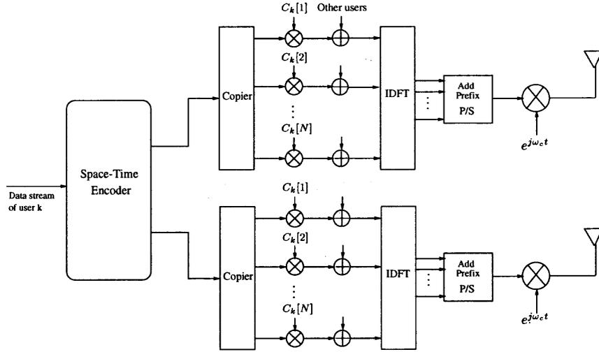
**Figure 3.1** A MC-CDMA transmitter with transmit diversity
