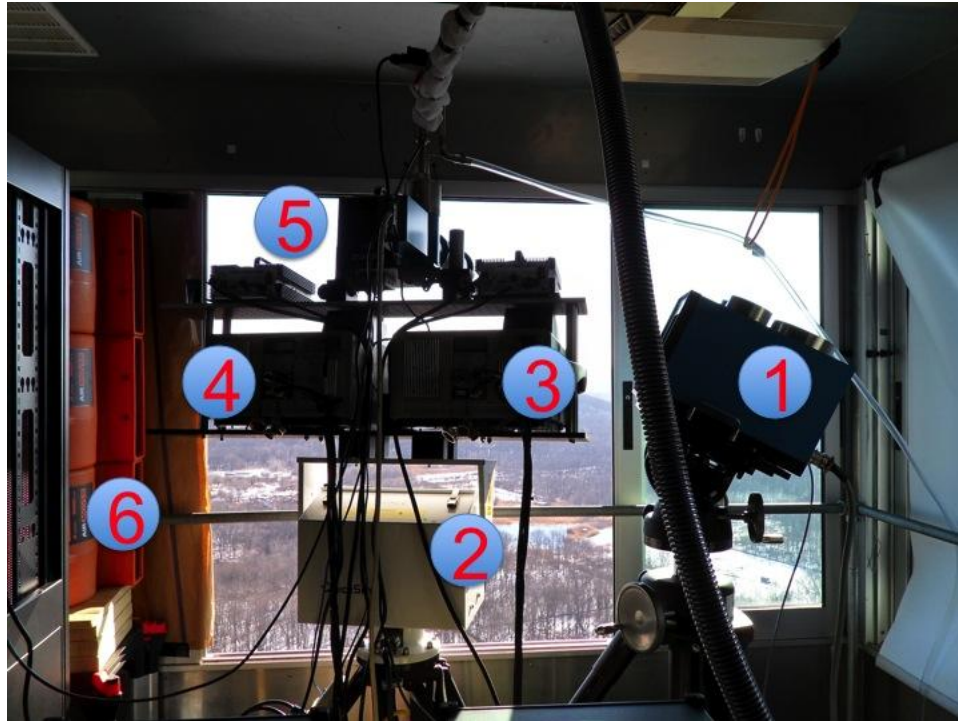
Figure 4.10 SPICE setup inside the facility elevator. Shown in the image is: 1) Mikron blackbody M350, 2) Quickset QTP-500 series, 3) Mid-Wave infrared hyperspectral Telops camera, 4) Long-Wave infrared hyperspectral Telops camera, 5) Long and Mid-Wave infrared polarimetric cameras from Polaris, 6) Blowers to protect sensors from rain and snow.
