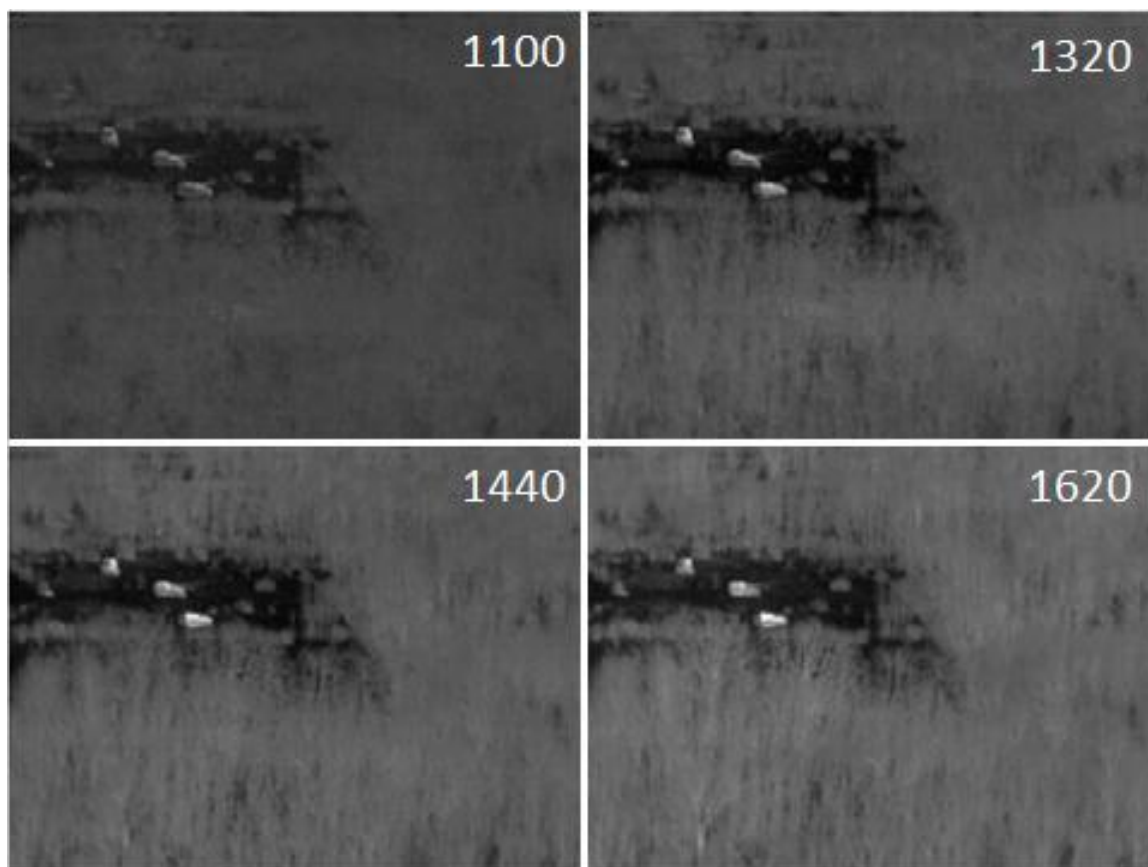
Figure 2.11 Example of high contrast scenarios using conventional LWIR imagery at different times in the day for 6 MAR 2010. Targets in the scene had the heating elements turned off. Continuous solar loading allowed the target plates to reach temperatures higher than the surrounding clutter.
