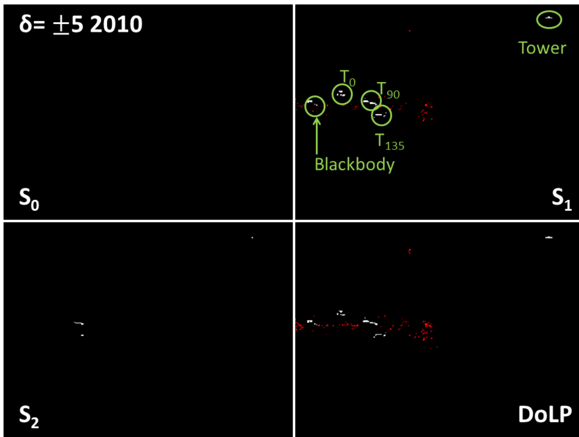
Figure 3.40 Output surfaces for S_0 , S_1 , S_2 , and DoLP using a common threshold value of \pm 5\sigma . As a result of the lack solar loading S_0 once again performed very poorly with virtually no manmade object detected for timestamp 2010h. S_1 , on the other hand, was able to identify all manmade objects in the scene with a lesser number of false alarms than DoLP. Conversely, DoLP was able to detect more pixels on the observation tower than S_1 imagery. S_2 successfully identified T_{90} and very small portions of T_{135} and the observation tower with no false alarms. However, T_0 and the external blackbody exhibited no strong S_2 polarization features that could be easily detected using the chosen threshold value.
