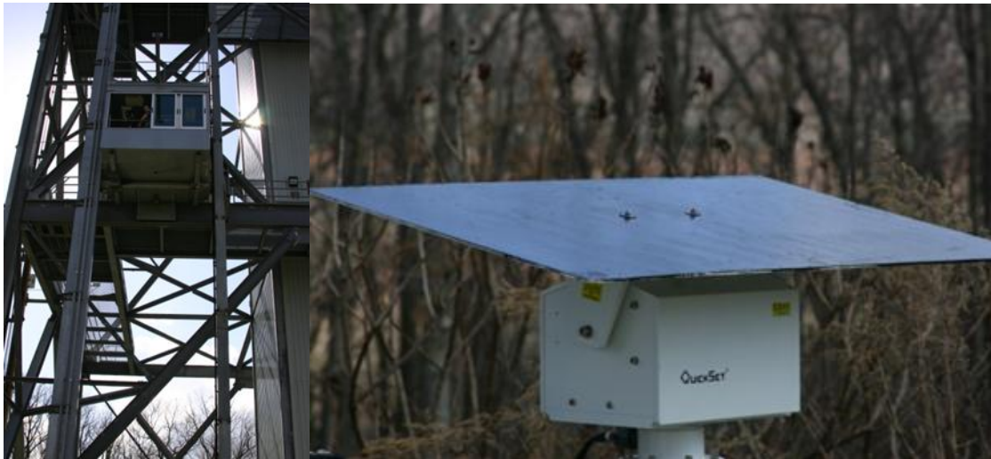
Figure 3.11 The Polaris LWIR polarimetric camera was located about 20 meters from the ground overlooking the test site. The test plate was placed on top of a pan and tilt system (QPT-500) and was tilted every five degrees from an initial position perpendicular to the camera (normal) to the final position parallel to the camera. The 0^\circ and 90^\circ intensity measurements were collected to represent the s and p -polarization components.
