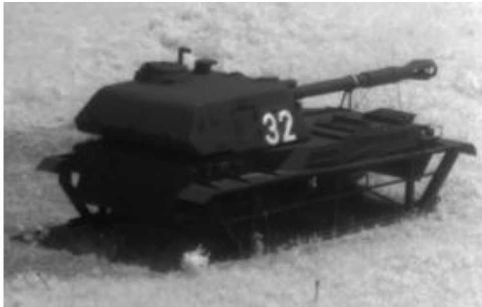
Figure 4.8 Surrogate target used in the SPICE data collection. At each of the mid and long range target sites, three targets were placed in different orientations, 0^\circ , 90^\circ , and 135^\circ with respect to the sensor.
