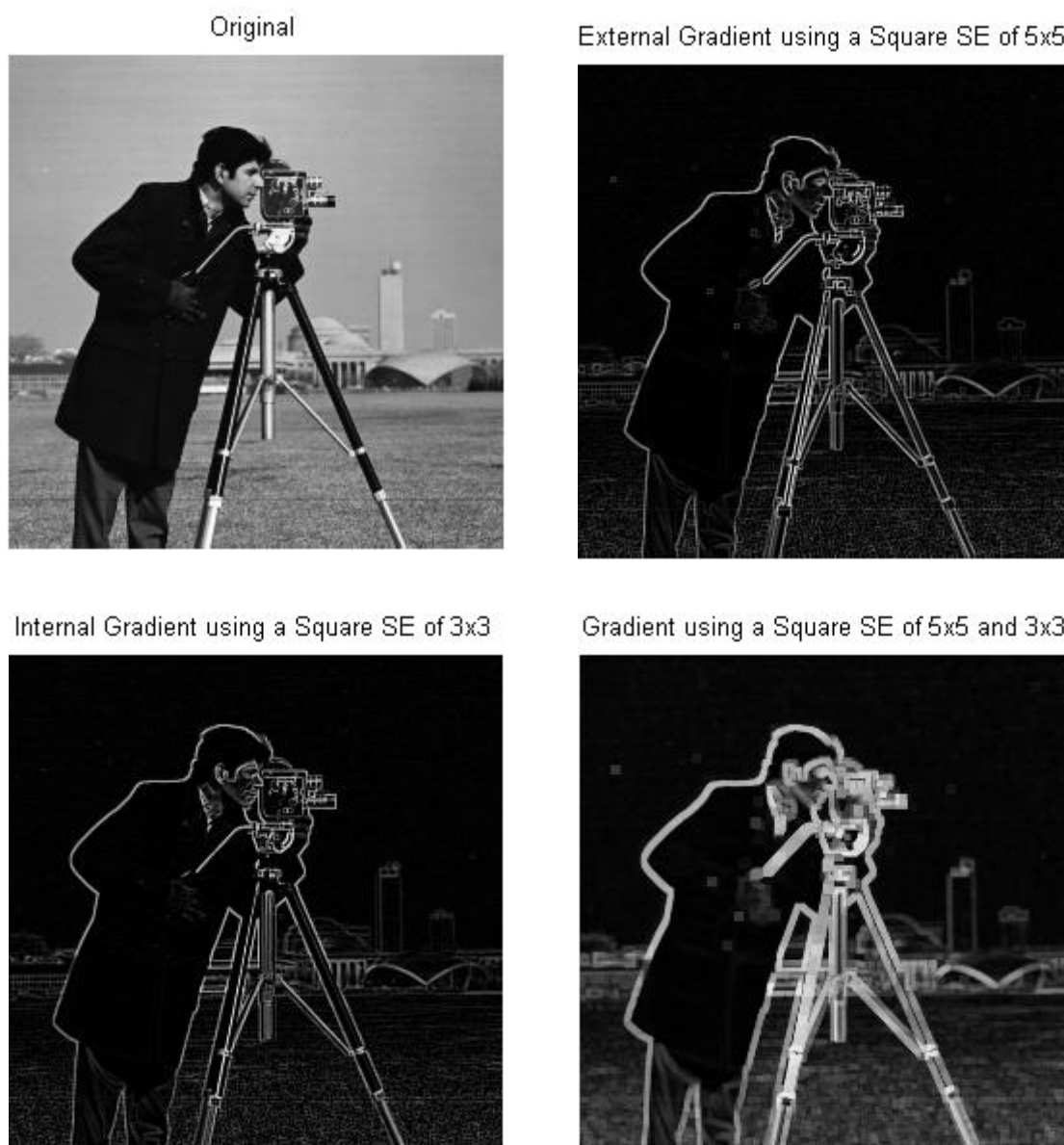
Figure 5.9 Illustration of using the gradient operator as a combination of the internal (upper right) and the external gradient (lower left) resulting on an effective edge detector (lower right) compared to top-hat transform.
