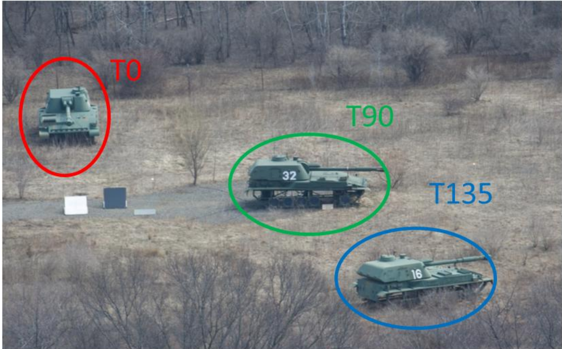
Figure 3.28 SPICE data collection surrogate targets placed at different viewing perspectives in relation to the data collection facility. The targets are designated by their respective angles (counterclockwise) as shown in the figure. The plates next to T_{90} were not present during the data collection presented in this dissertation.
