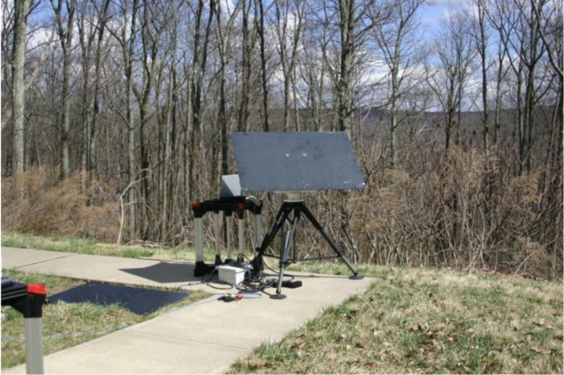
Figure 3.12 View of the plate on the pan and tilt system (QPT-500). In the test scene there are three manmade objects present, the test plate on the QPT-500, the reference plate on the floor, and the sidewalk. Grass is the predominant clutter class found in the sensor's field of view.
