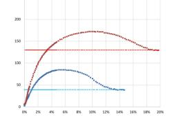
Figure 1: Deviator stress curves for sample 1 and 2
