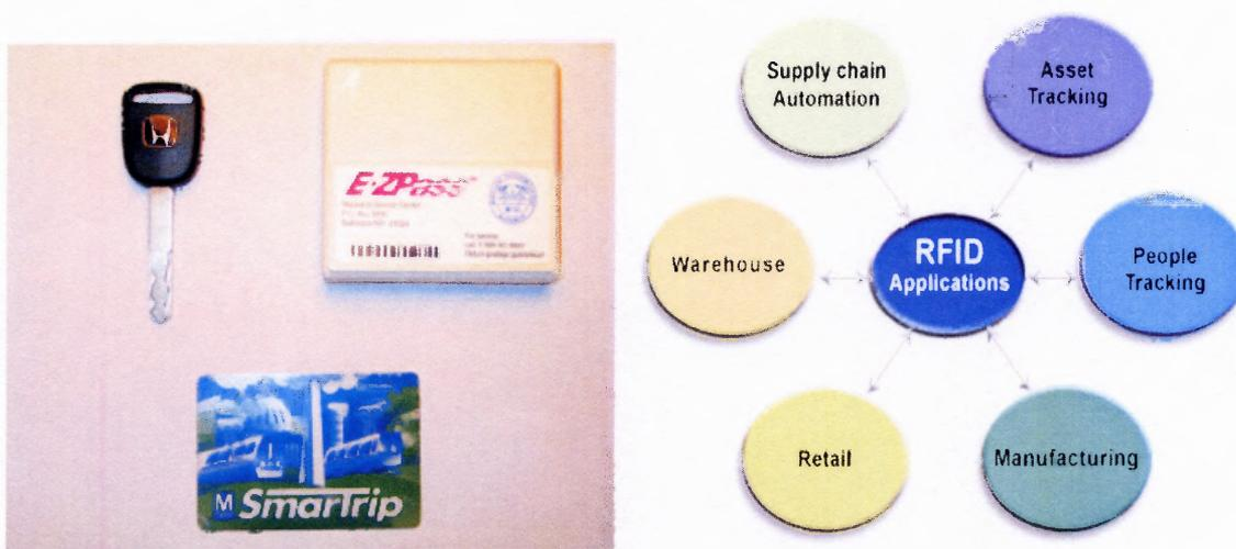
**Figure 2.9** Application of RFID and some of the daily use RFID equipments.
