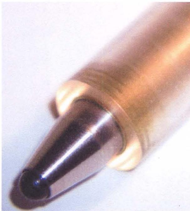
**Figure 3.8** Lightpipe illuminator.
