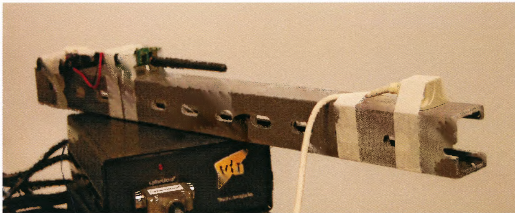
Figure 6.5 Experimental setup showing the IMU and FOB on a beam.
