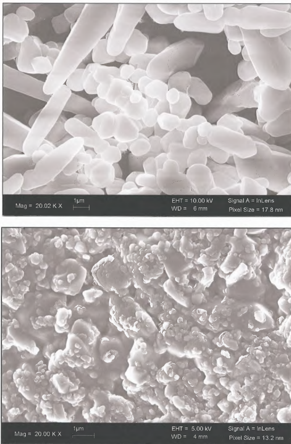
Figure 4.23 SEM Micrographs of the griseofulvin particles before milling (top) and after milling with sodium alginate (bottom).
