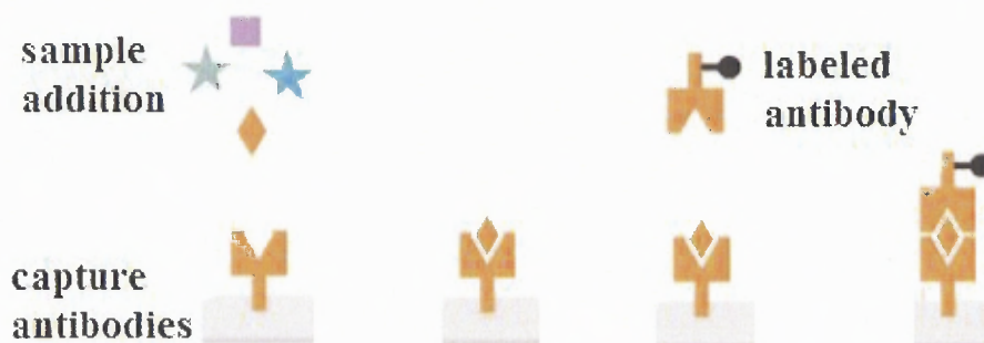
Figure 2.2 Schematic of label-based technique for immunosensing.
