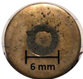
Figure 2.3 Brass sample holder used in ESD experiments with surface coated with residue produced after an ignition event.
