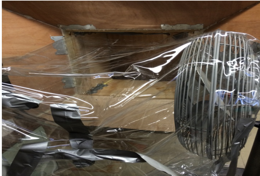
Figure 5.1 An electric fan connected to the suction with plastic foils at the entrance of the wind tunnel, serving as wind source.
