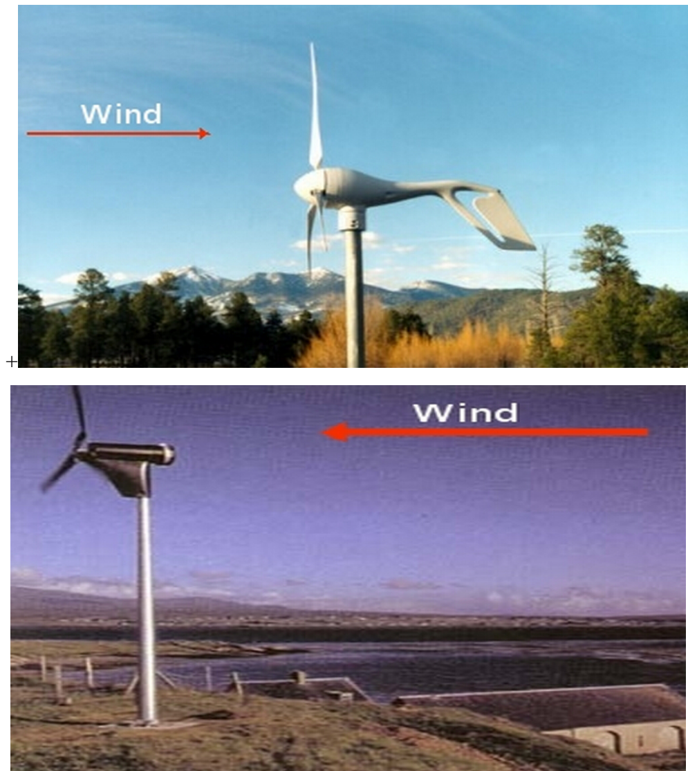
Figure 4.5 Upwind (upper) and downwind (lower) design of wind turbine rotor. Source: Upwind Turbine Vs. Downwind, http://www.power-talk.net/upwind-turbine.html . Accessed 04/20/2015.
