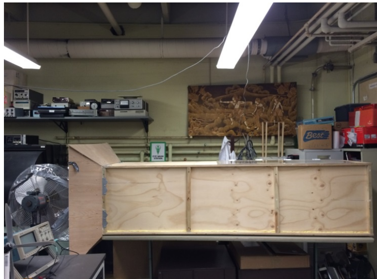
Figure 4.7 The wind tunnel used for wind turbine experiments.
