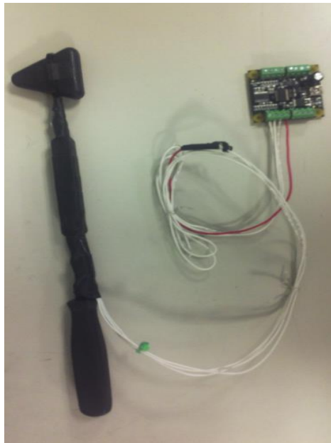
Figure 2.1 figure showing the instrumented hammer.
