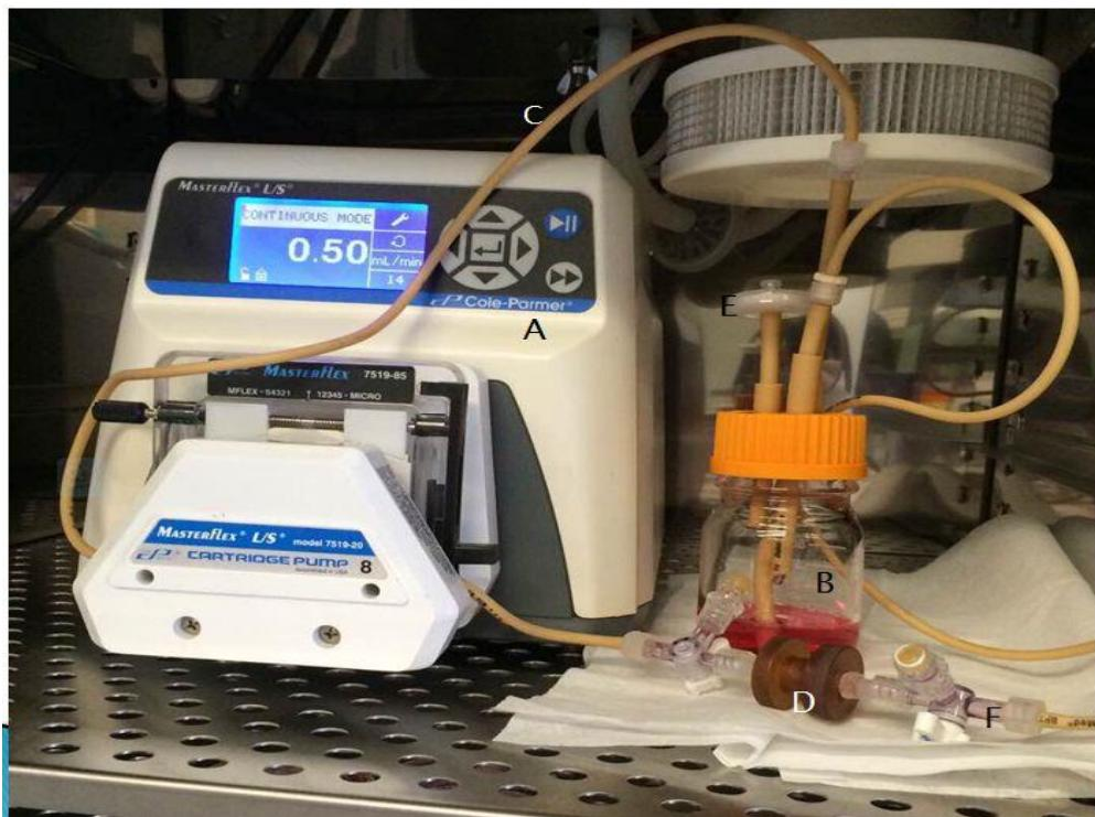
**Figure 3.2** Flow bioreactor system. A flow bioreactor system consists of (A) a peristaltic pump, (B) a media reservoir, (C) L13 sized tubing, (D) a bioreactor chamber housing a 3D collagen tissue . (E) a  $0.2\text{ }\mu\text{m}$  air filter for gas exchange and (F) a 3-way stop-cock/injection port for medium exchange.
