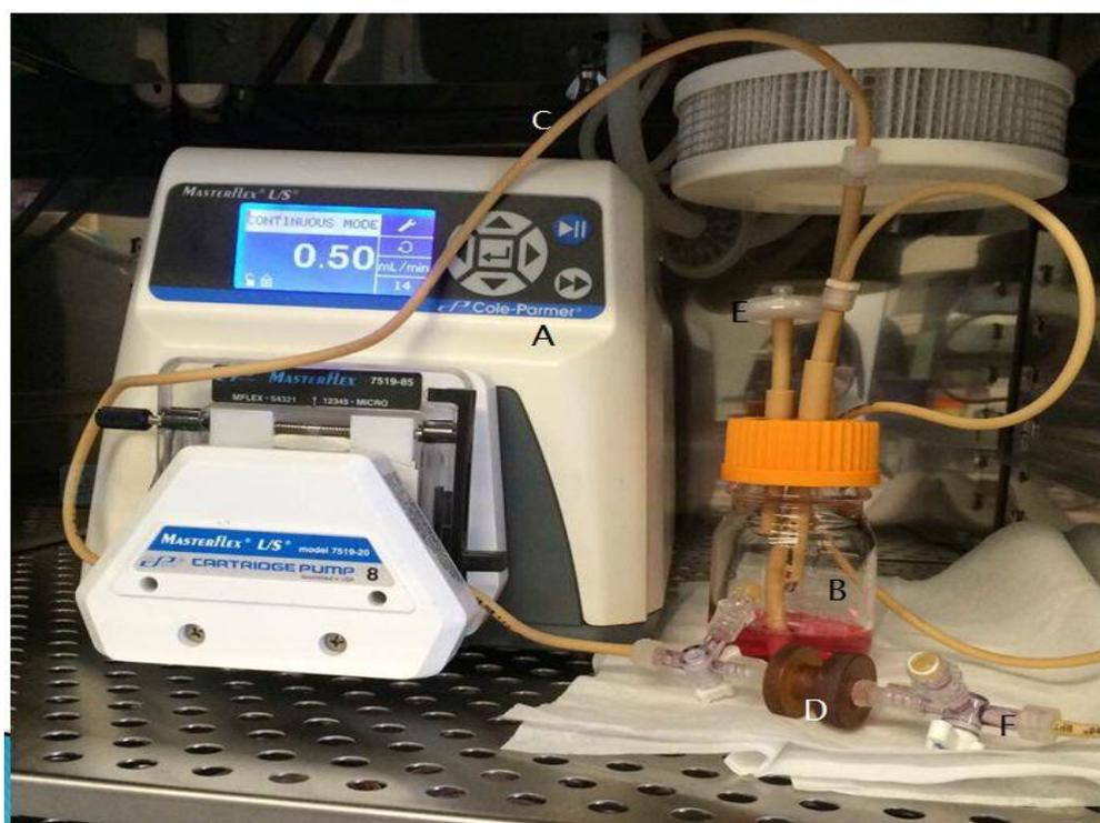
**Figure 3.2** Flow bioreactor system. A flow bioreactor system consists of (A) a peristaltic pump, (B) a media reservoir, (C) L13 sized tubing, (D) a bioreactor chamber housing a 3D collagen tissue. (E) a 0.2  $\mu\text{m}$  air filter for gas exchange and (F) a 3-way stop-cock/injection port for medium exchange.
