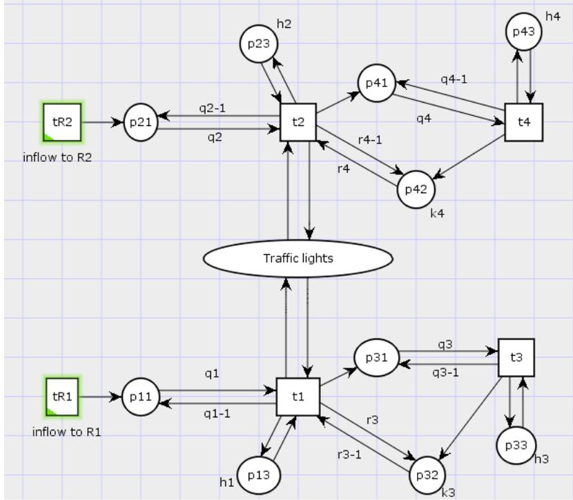
**Fig. 4.3** Intersection modeled by a continuous PN
