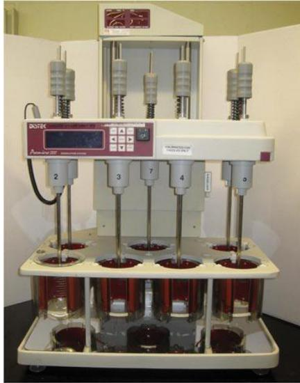
**Figure 2.1** Distek Premiere 5100 dissolution system used in this work.
