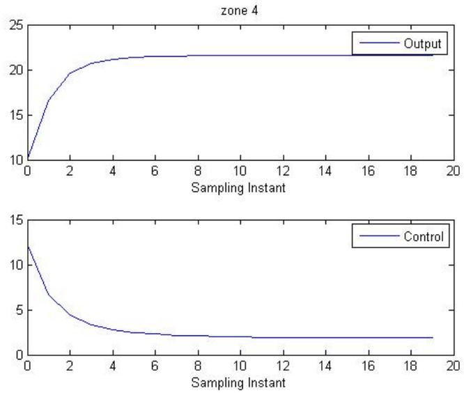
**Figure 6.5** Simulation without heat transfer of zone 4.
