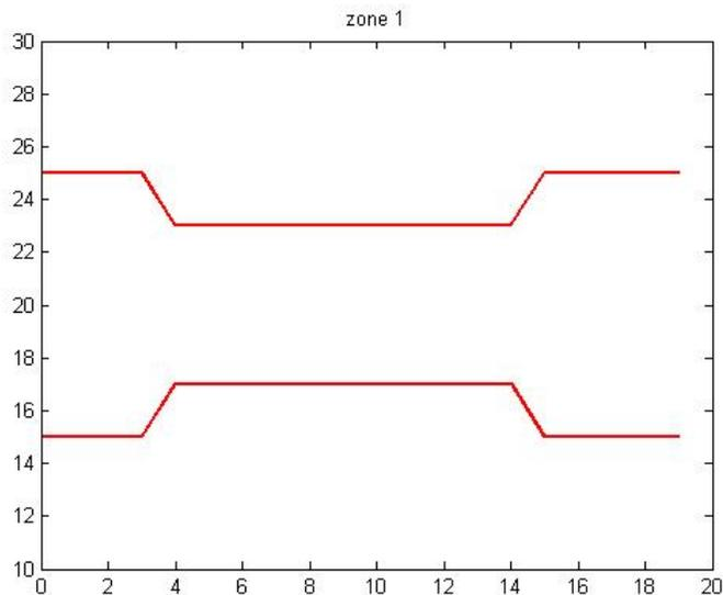
**Figure 8.5** Constraint of temperature of zone 1.
