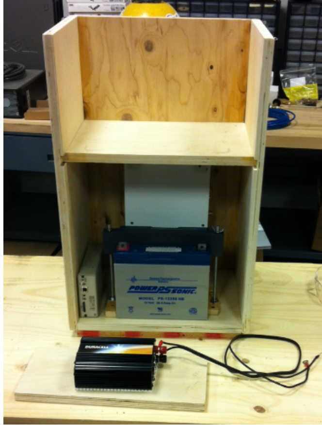
Figure 2.1 Unassembled HAMPRE (trakSTART™, DATAQ, battery, and inverter)
