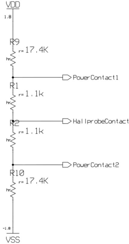
**Figure 4.5** The equivalent circuit of the circular VHD.
