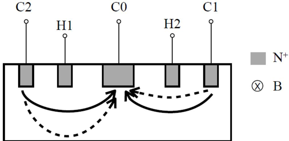
**Figure 2.5** The vertical Hall Plate has three Power contacts and two Hall probe contacts. C1 and C2 are connected with VDD, and C0 is connected with GND. Current will flow from C1 and C2 to C0. H1 and H2 are used to detect the variation of current caused by the magnetic field.
