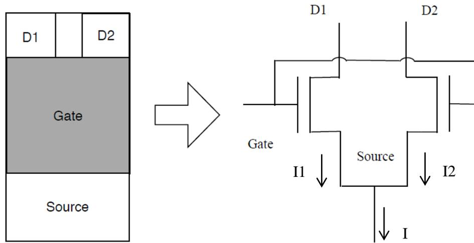
**Figure 4.1** The equivalent circuit of the SD-MAGFET.
