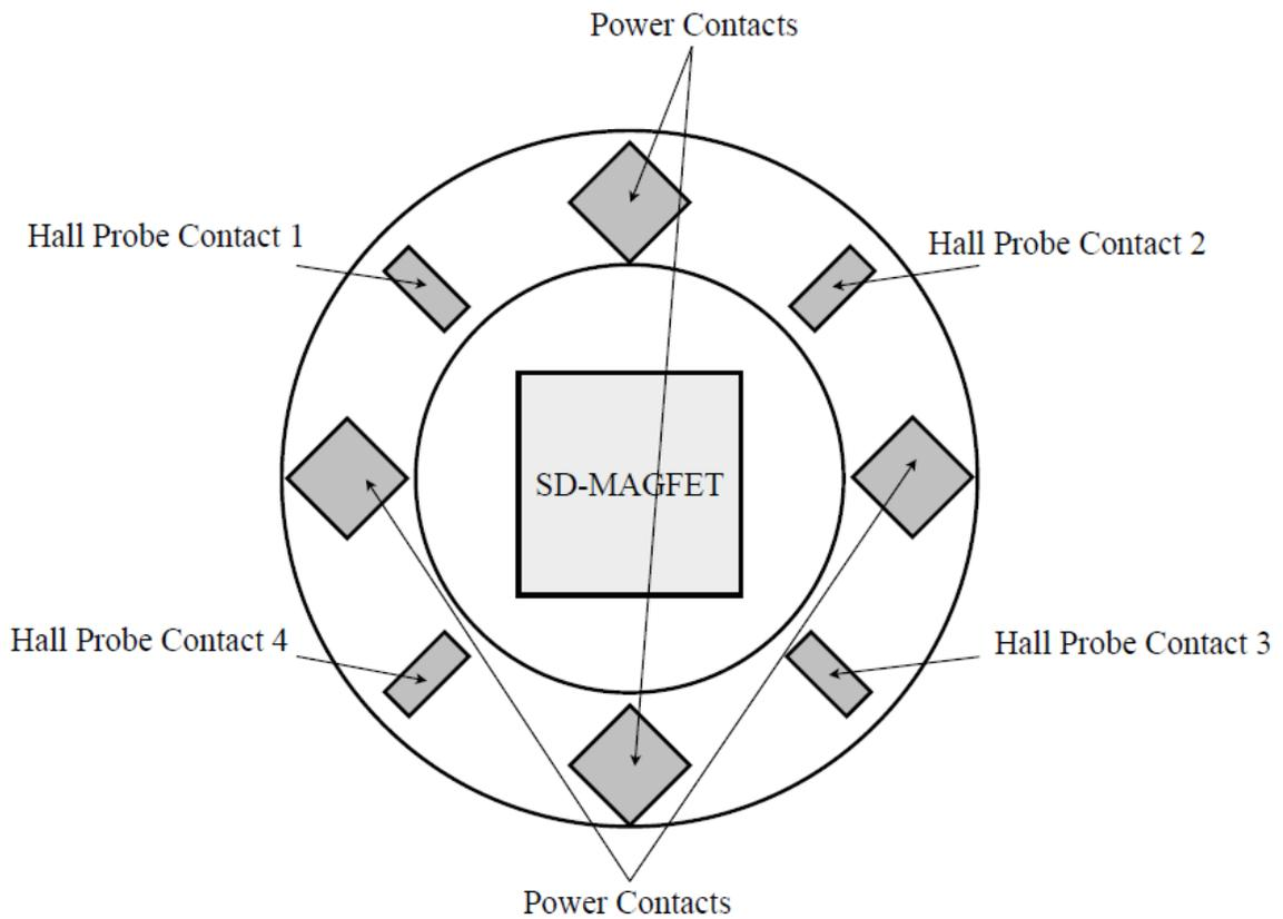
**Figure 3.6** The entire pattern of the three-dimensional MFS is shown in this figure. The SD-MEGFET which has the independent power supply is located at the center of the device. The detail of the circular VHD located around the SD-MAGFET is also shown in this figure.
