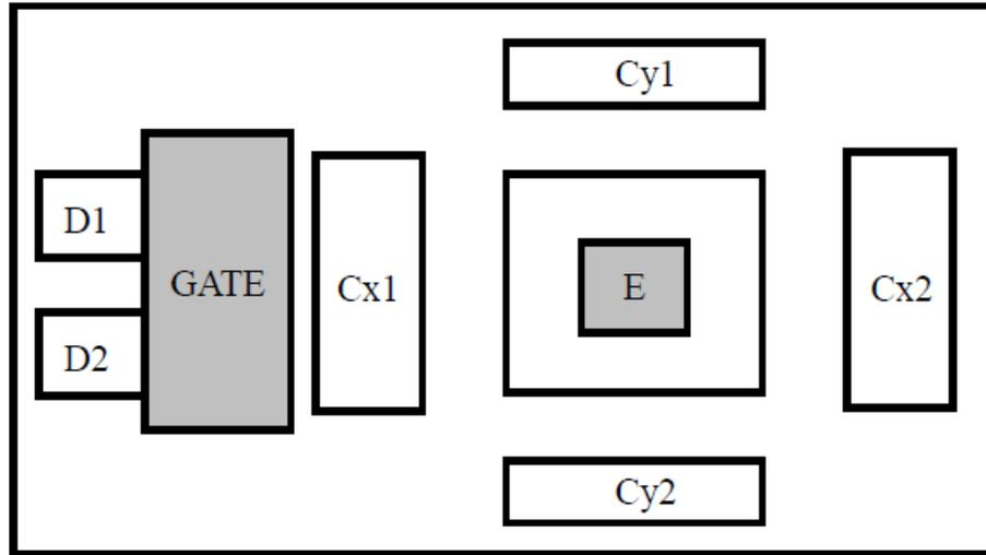
**Figure 2.11** The three-dimensional MFS in BiCMOS technology adapted from [11].
