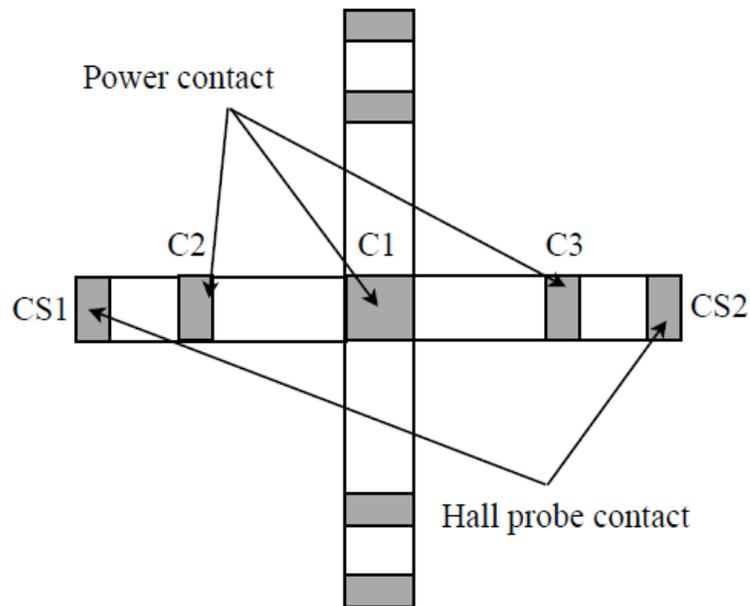
**Figure 2.7** The bar-shaped two-dimensional MFS adapted from [7].
