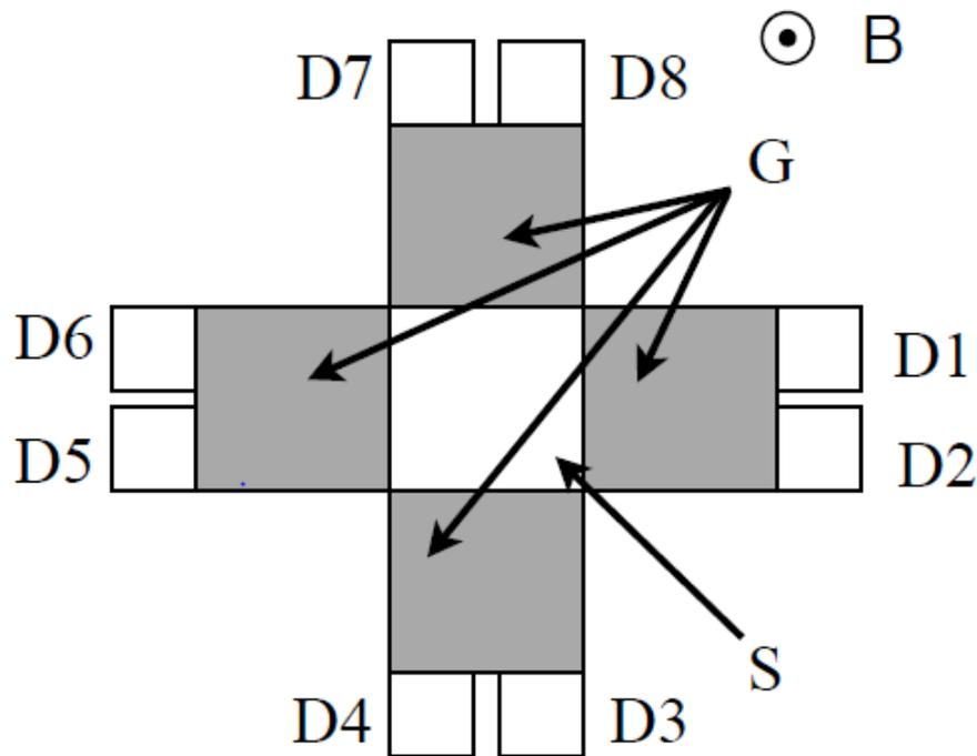
**Figure 3.2** Four SD-MAGFETs with a common source connection.
