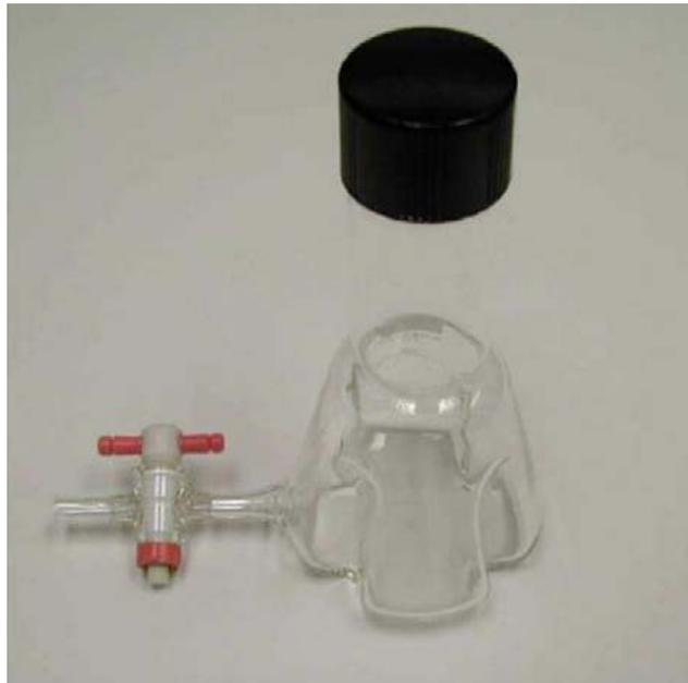
**Figure 2.1** Photograph of a baffled trypsinizing flask.
