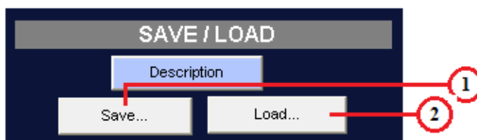
Figure 4.8 Labeled view of the Save / load panel.
