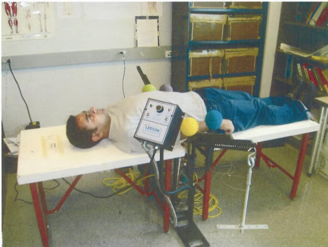
**Figure 3.1** Subject on the automated anatomic torsion monitor (A-ATM).
