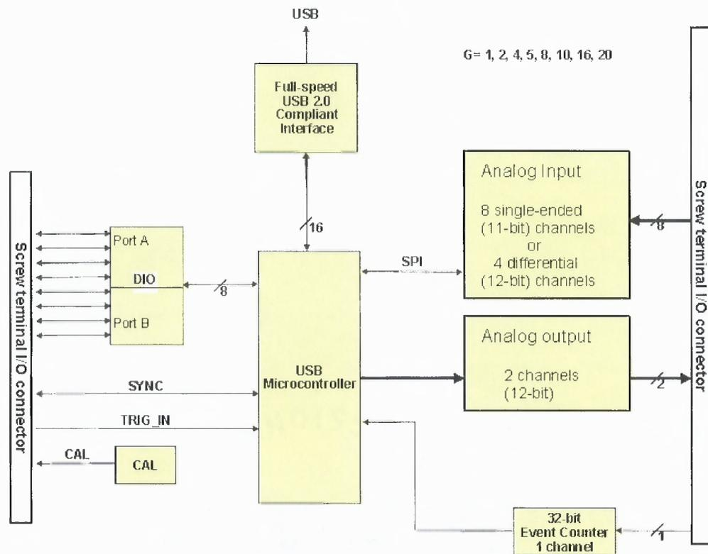
**Figure 2.7** Block diagram for DAQ card.
