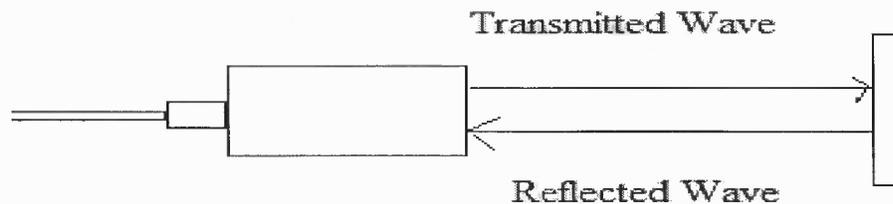
**Figure 2.2** Working of ultrasonic sensors.
