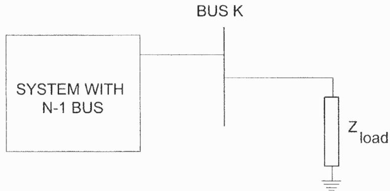
**Figure 4.1** System for Calculating Z-thevenin at Bus K.
