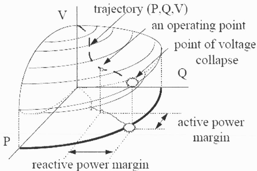
**Figure 1.2** Voltage – Power diagram including reactive power.
