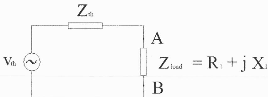
**Figure 4.2** Thevenin Equivalent Circuit for System in Figure 4.1.
