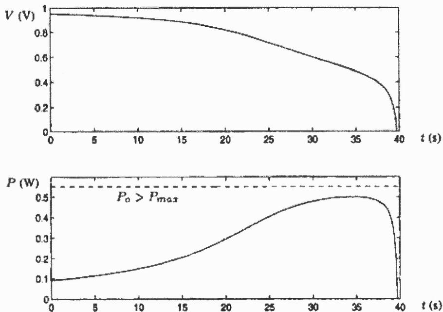
**Figure 3.7** Voltage instability in a DC system, source [5].
